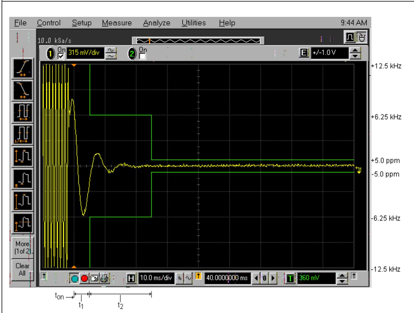
**Plot 5.12.4.2. Transient Frequency Behavior for 12.5 kHz Channel Spacing**
