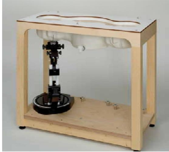
For Head mounted devices placed next to the ear, the phantom used in the evaluation of the RF exposure of the user of the wireless device is an IEEE P1528 compliant SAM Twin phantom, shaped like a human head and filled with a mixture simulating the dielectric characteristics of the brain. A left sided head and a right sided head are evaluated to determine the worst case orientation for SAR.
