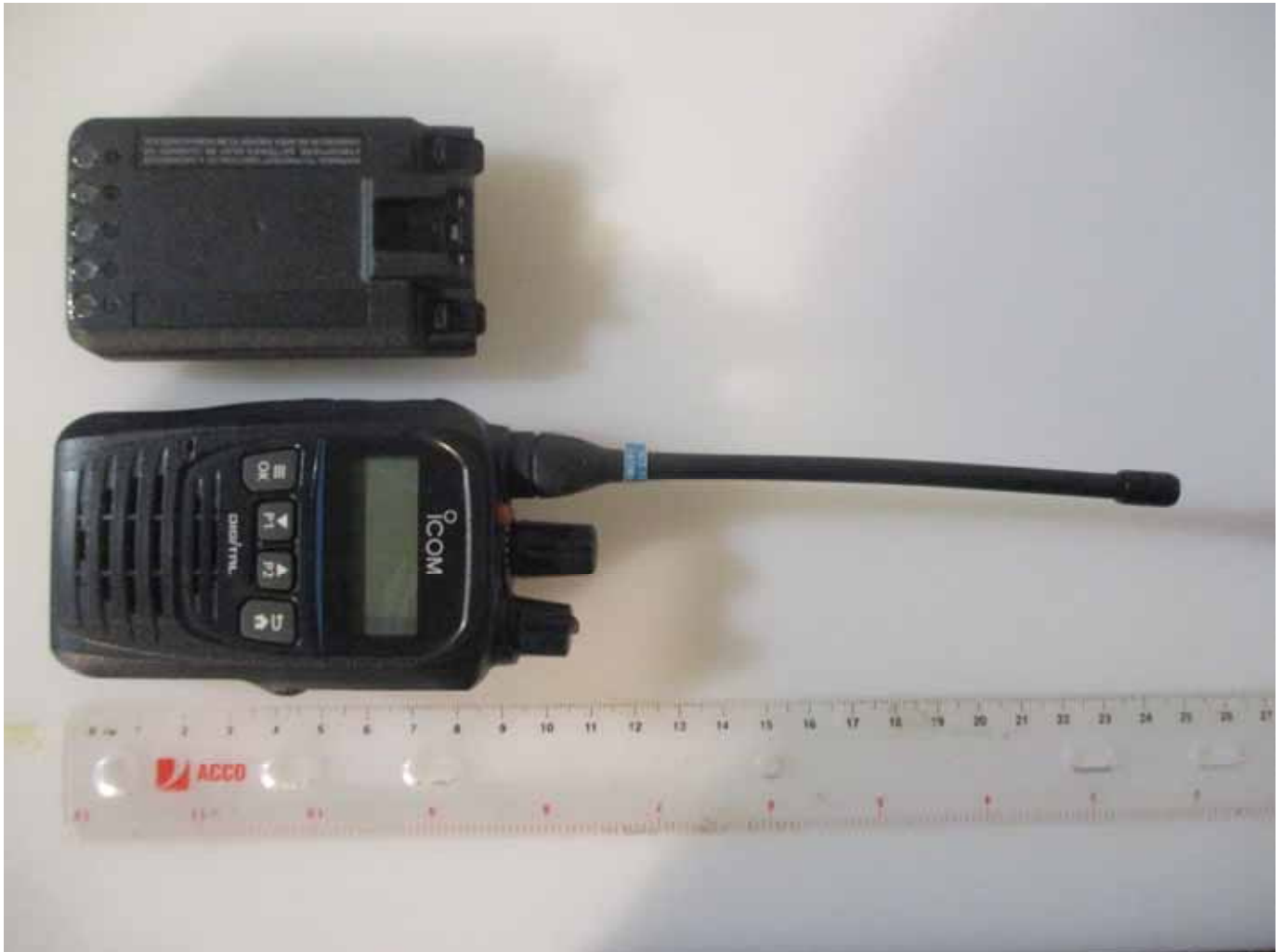
< D.U.T.'s front view with battery and FA-S61UC Cut Antenna 460MHz 142mm >
