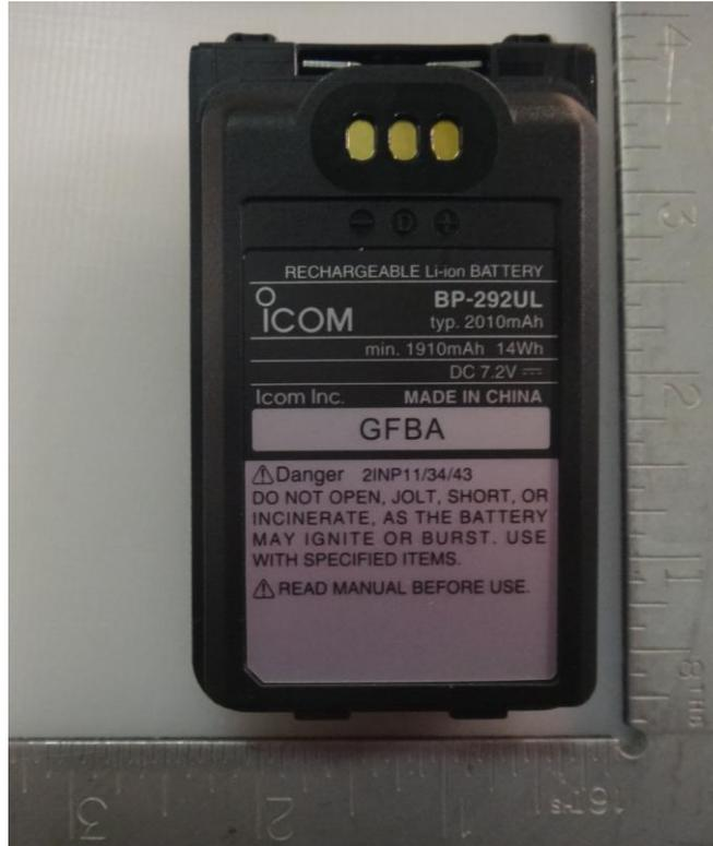
*Li-ion Chargeable Battery (M/N: BP-292UL, 7.2V, 2010mAh)*
