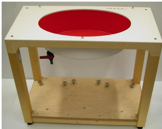
For body mounted and frontal held push-to-talk devices, an IEC 62209-2 compliant Oval Flat Phantom (ELI 4.0) with a base plate thickness of 2mm is used.
