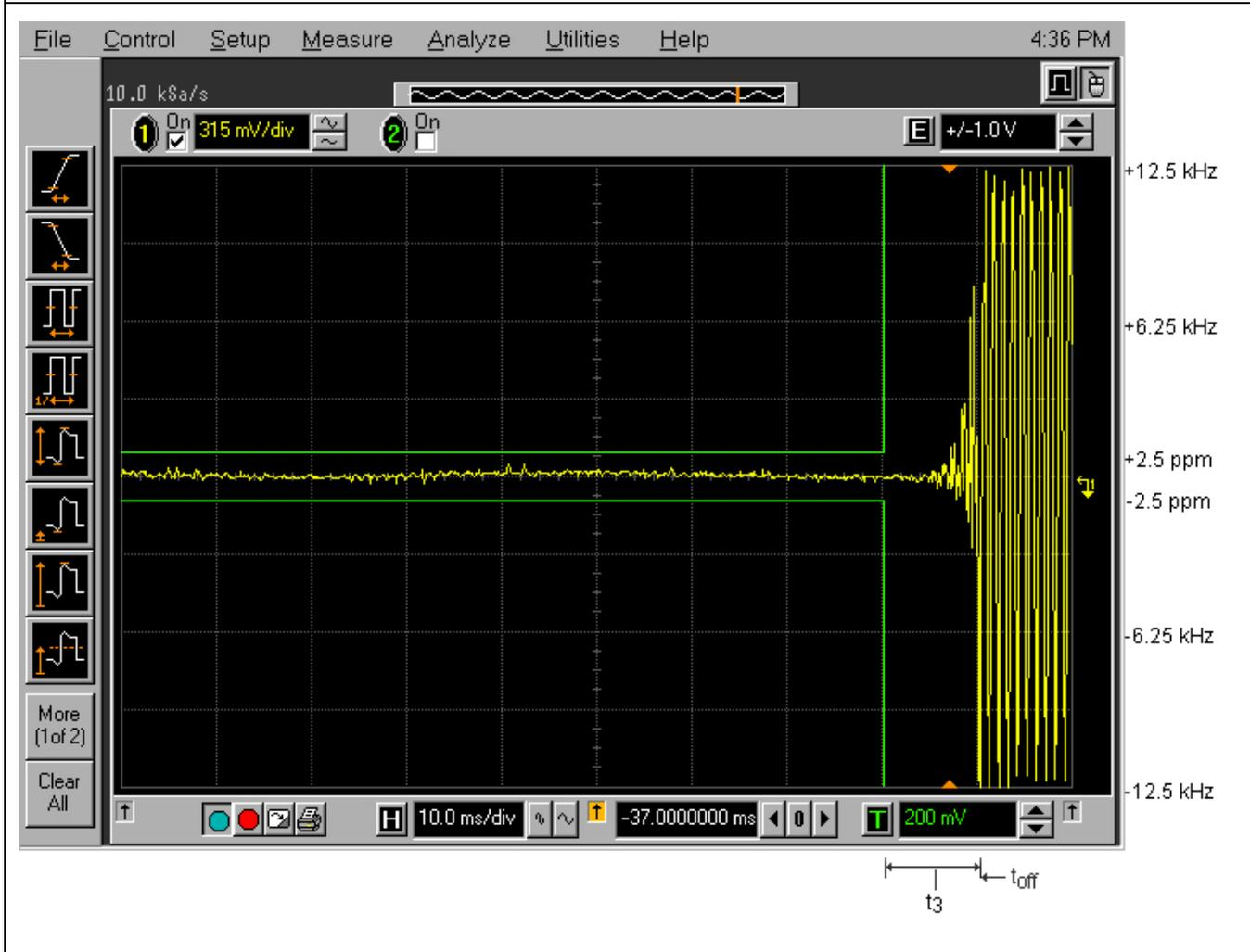
Plot 5.12.4.3. Transient Frequency Behavior for 25 kHz Channel Spacing
