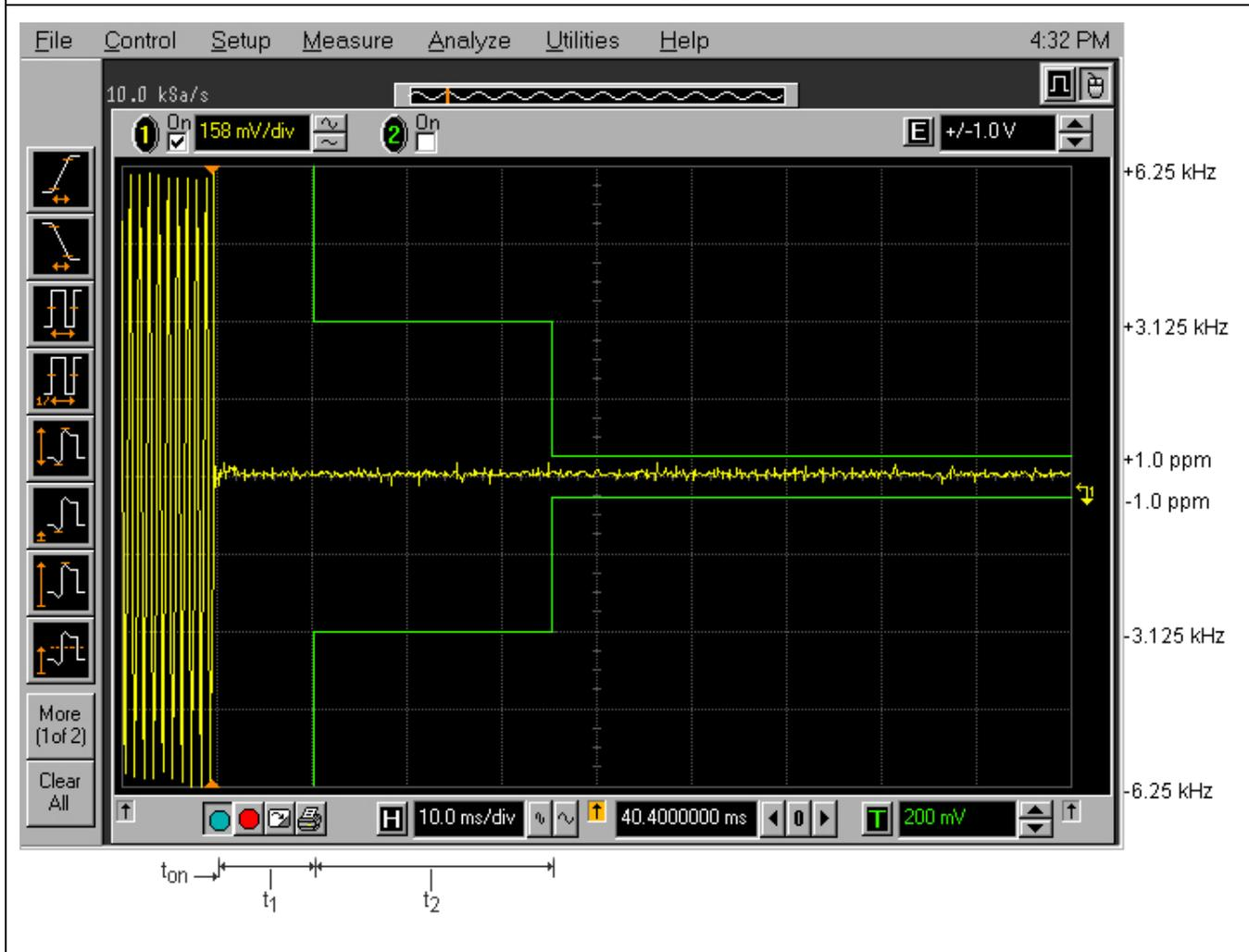
Plot 5.12.4.6. Transient Frequency Behavior for 6.25 kHz Channel Spacing
