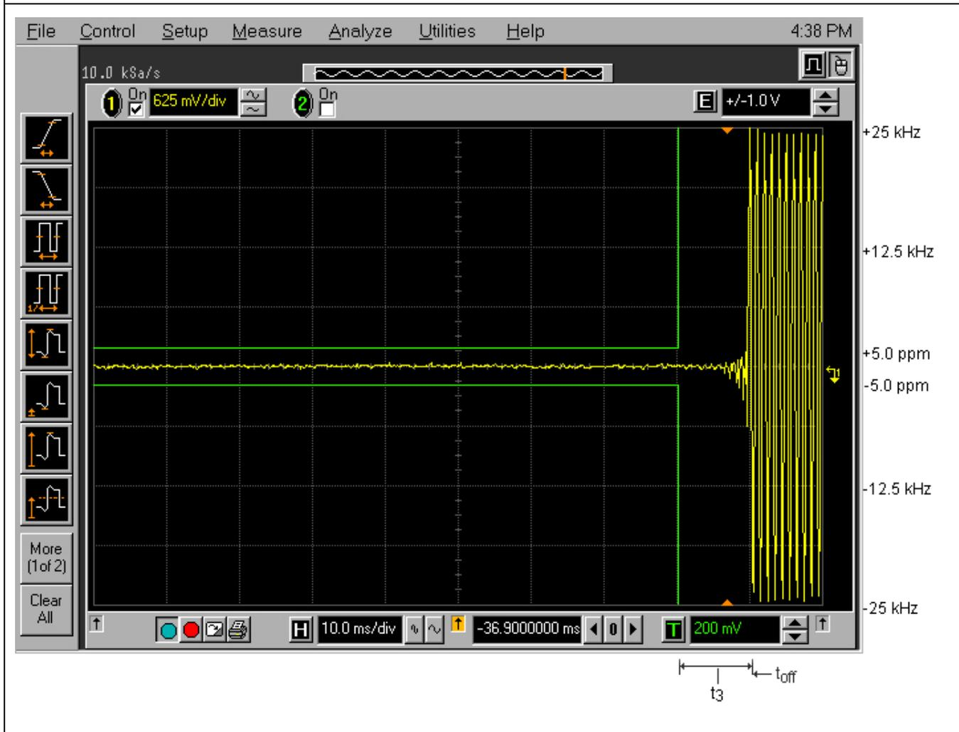
Plot 5.12.4.5. Transient Frequency Behavior for 6.25 kHz Channel Spacing
