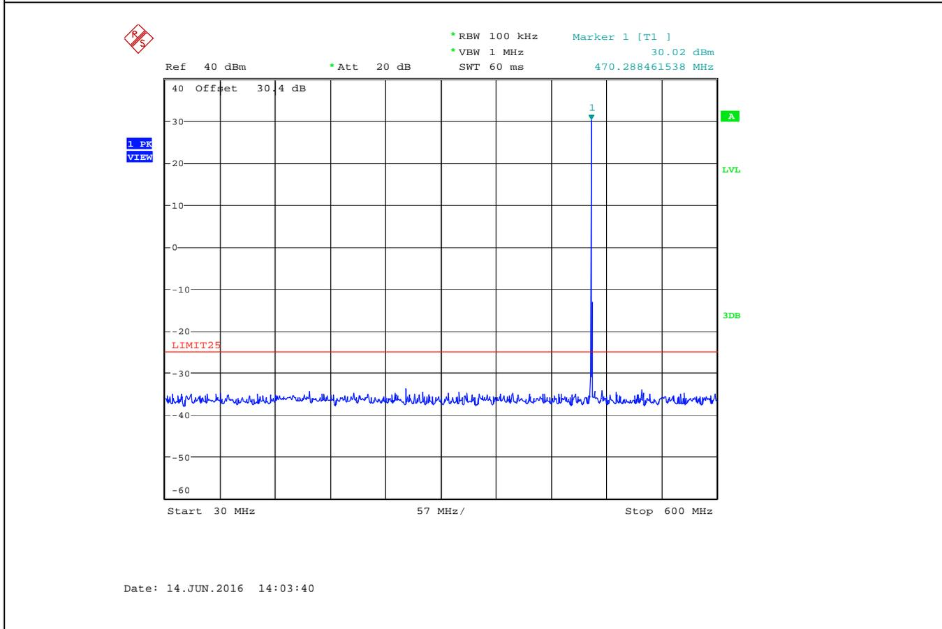
Plot 5.9.4.3.4. Conducted Transmitter Spurious Emissions for 469.975 MHz, Low Power, 600 MHz - 5 GHz
