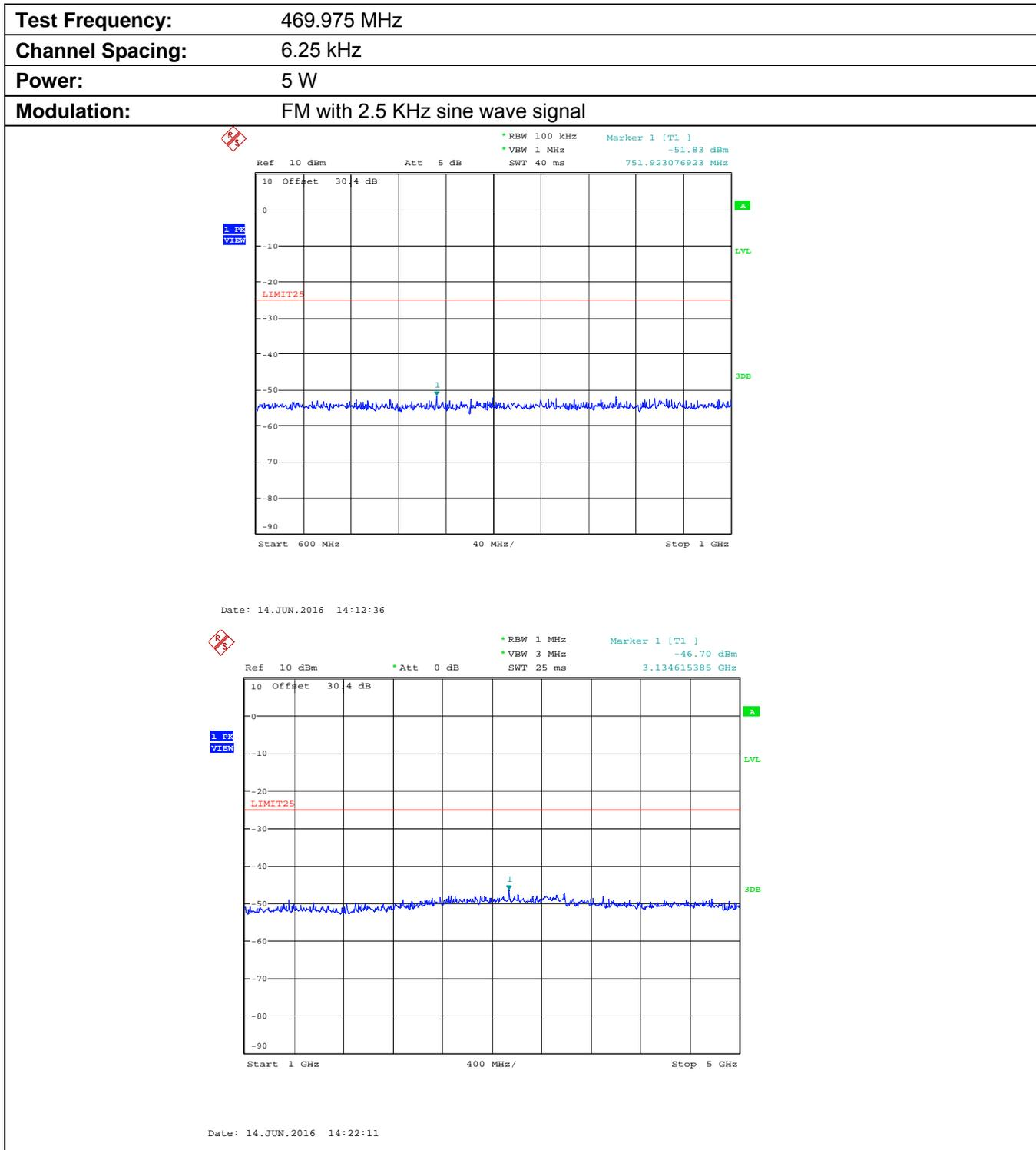
Plot 5.9.4.3.3. Conducted Transmitter Spurious Emissions for 469.975 MHz, Low Power, 30 MHz - 600 MHz
