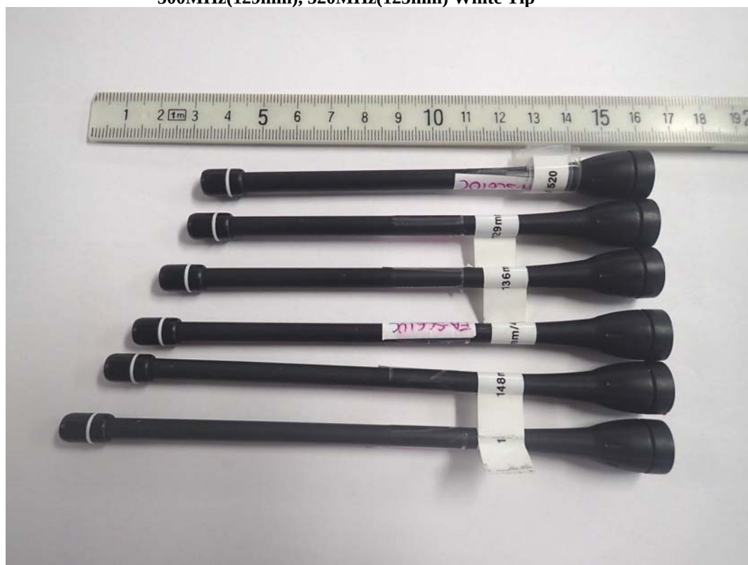
Cut Antenna FA-SC61UC 420MHz (156mm), 440MHz (148mm), 460MHz (142mm), 480MHz (136mm), 500MHz(129mm), 520MHz(125mm) White Tip
