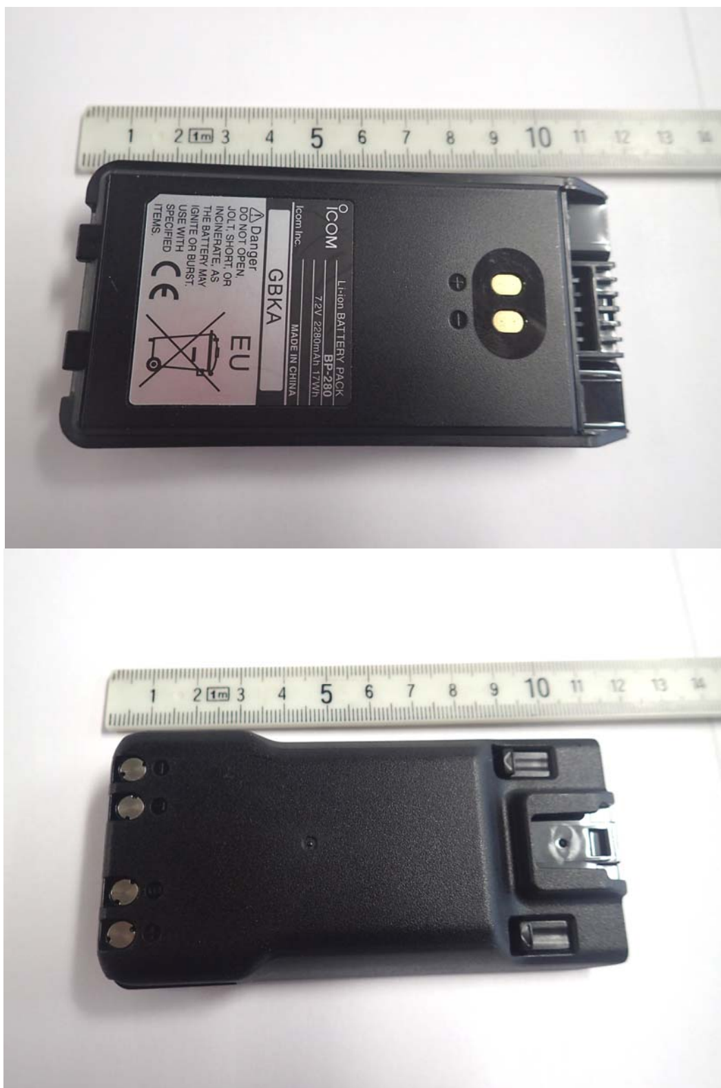
(Li-ion Chargeable Battery (M/N: BP-280 Li-ion, 7.2V, 2280mAh))
