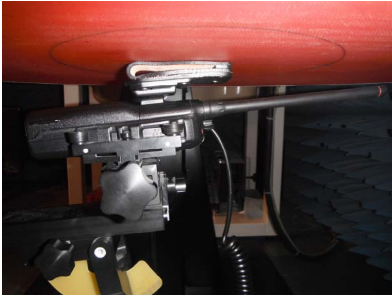
Back side of EUT in parallel to the phantom with the belt-clip (M/N: MB-96) in contact, attached HM-184 Speaker Microphone
