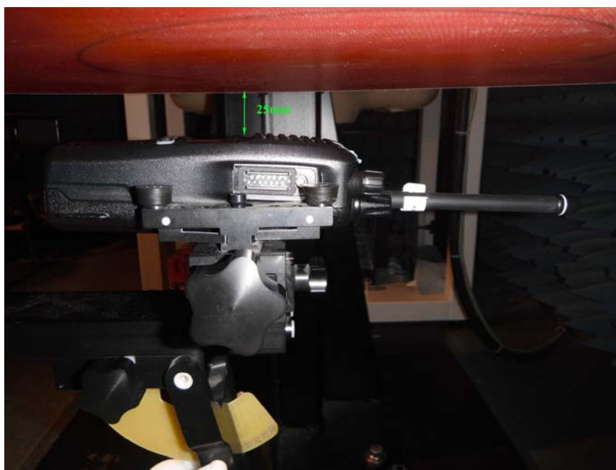
< FA-SC61VC cut antenna with the length of 133mm >
