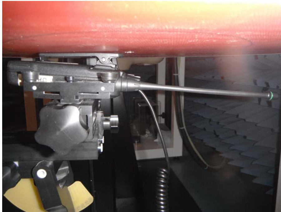
Back side of EUT in parallel to the phantom with the belt-clip (M/N: MB-133) in contact, attached HS-158LA Speaker Microphone
