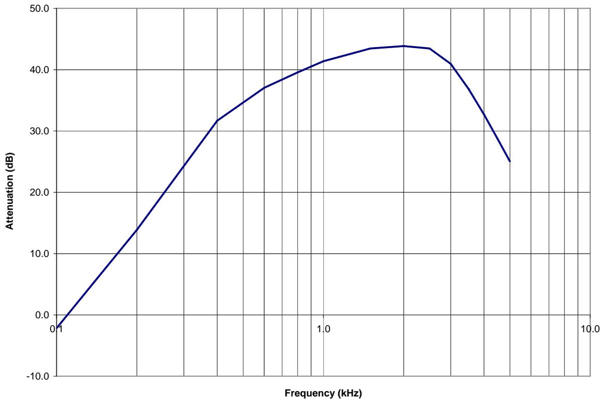
Audio Frequency Response- Attenuation w.r.t 1kHz
