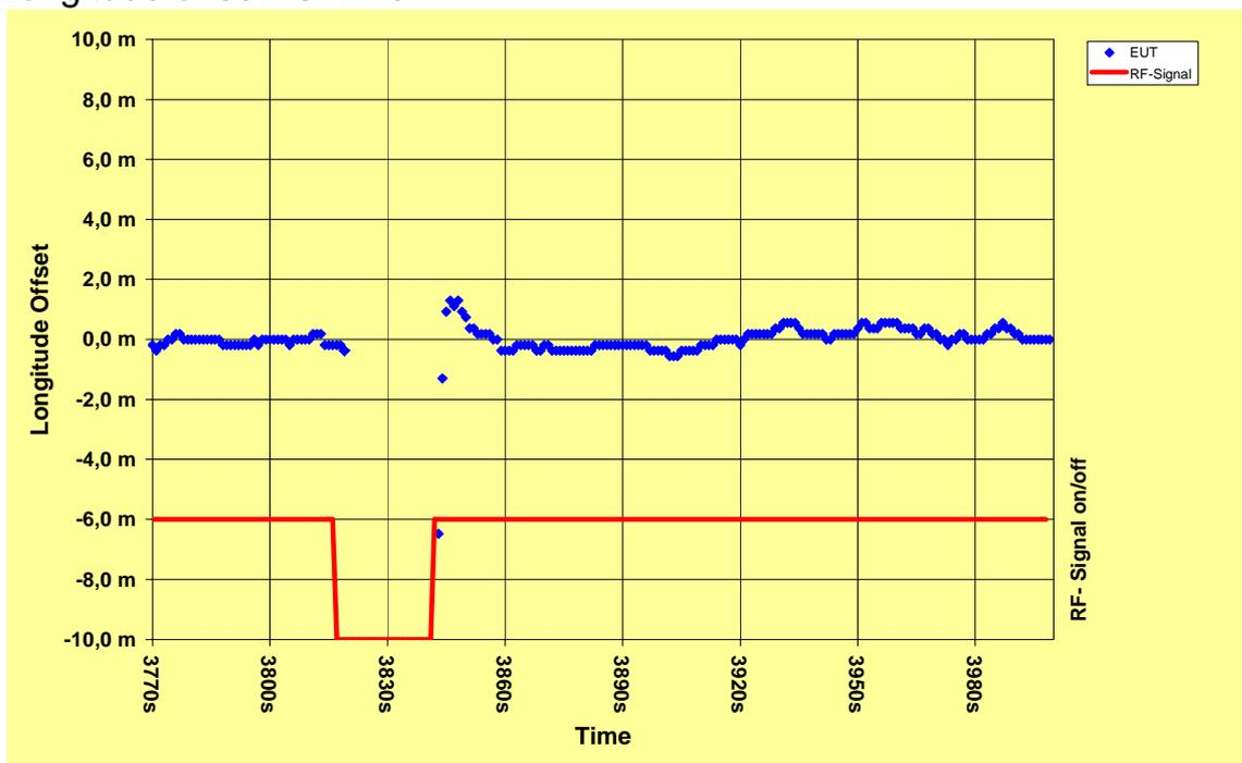
Position offset after time limit of 30seconds after restored RF signal
