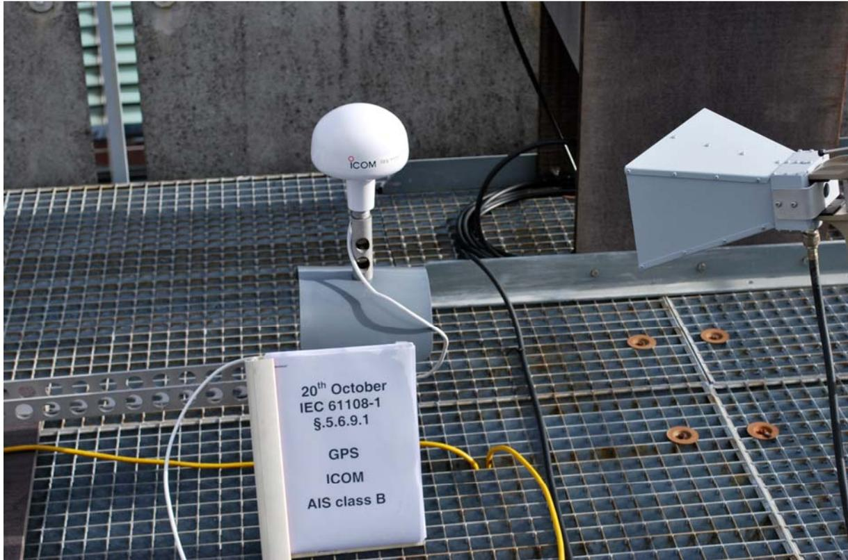
**EUT – S –Band interference test**
