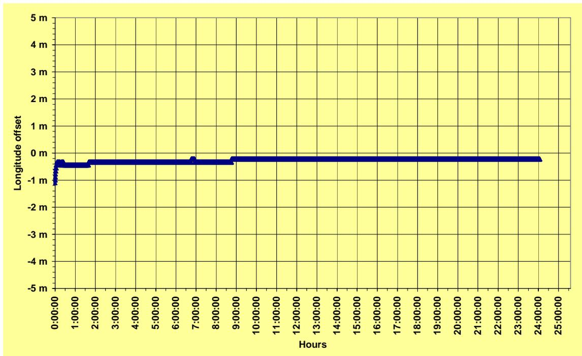
Position offset – GPS static accuracy
