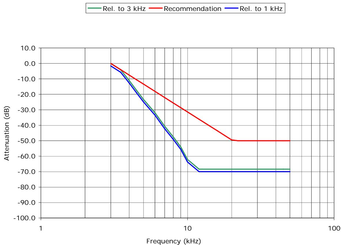
**5.7.4.2. 25 KHz Channel Spacing, F3E, Frequency of All Modulation States\***
