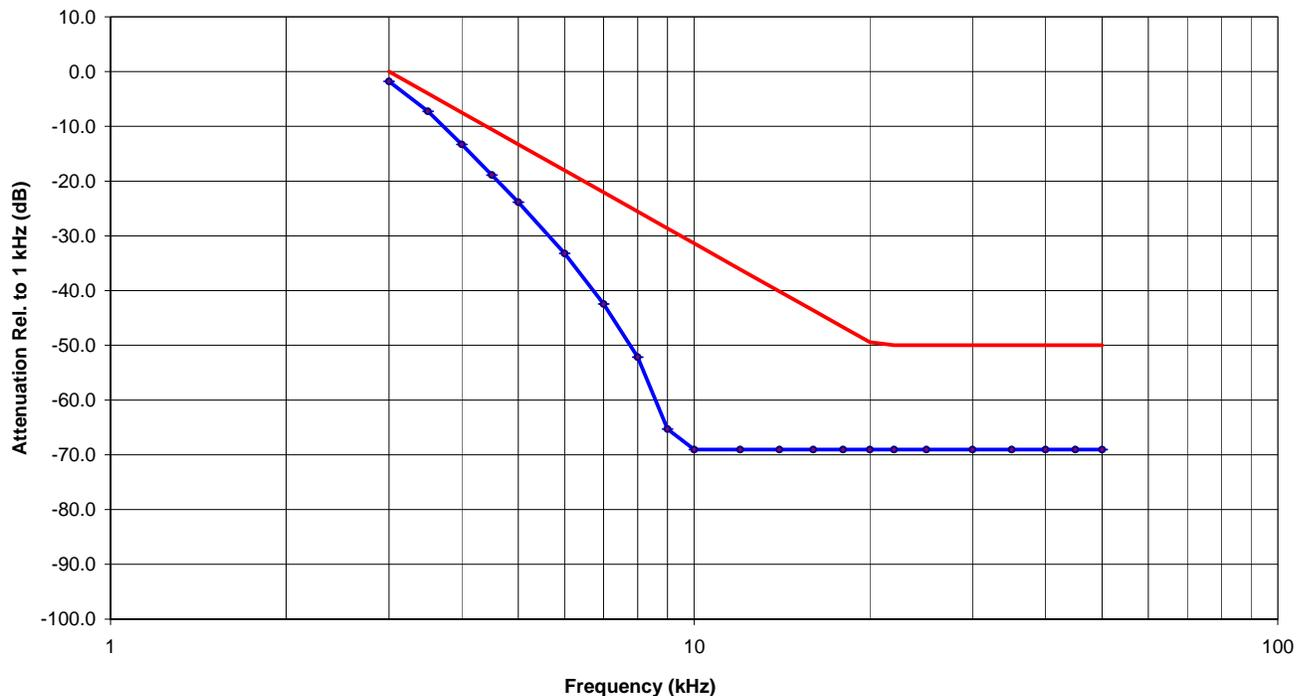
**6.7.5.2. 25 KHz Channel Spacing, F3E, Frequency of All Modulation States\***
