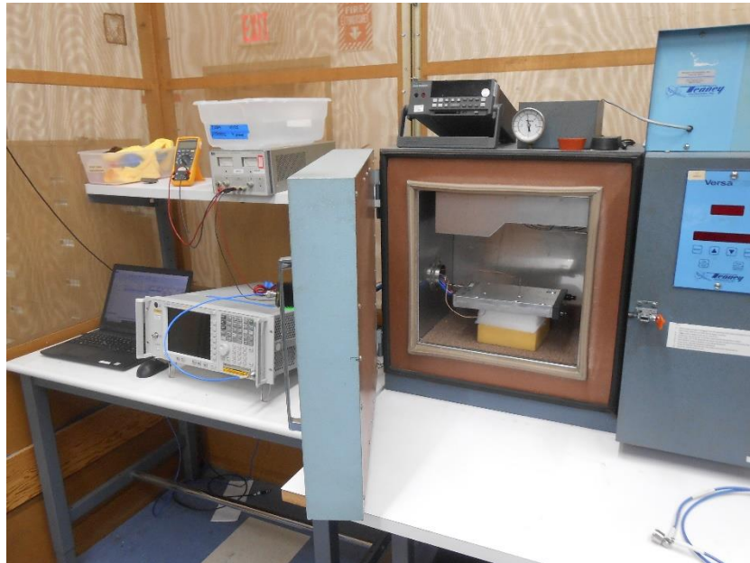
Frequency Stability Test Setup 1
