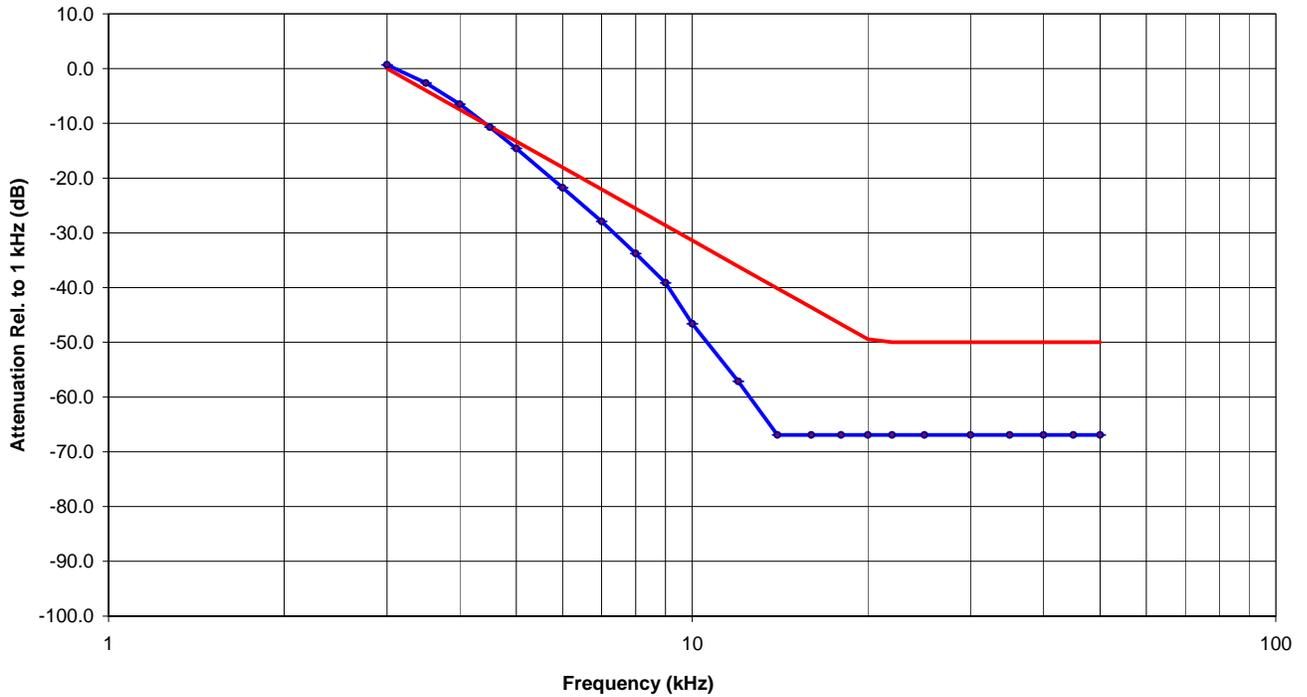
**6.7.5.2. 25 KHz Channel Spacing, F3E, Frequency of All Modulation States\***
