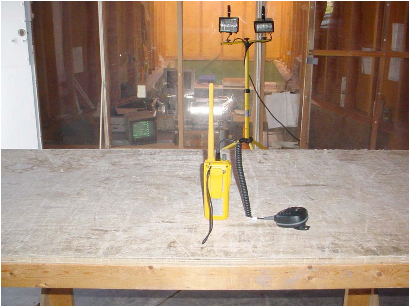
Radiated Emissions Orthogonal Position #1
