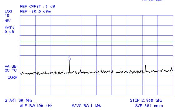
Plot # 4: Receiver Antenna Port Power Conducted Emissions
