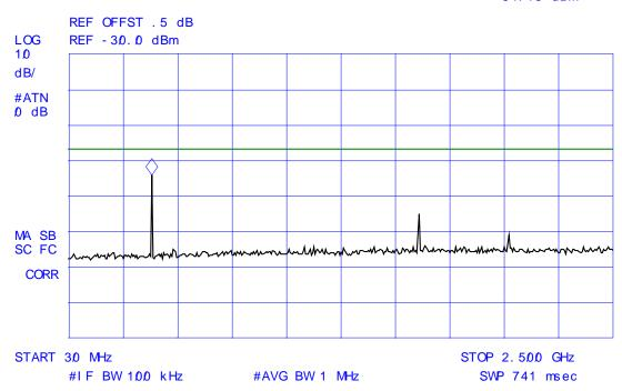
Plot # 3: **Receiver Antenna Port Power Conducted Emissions Receive Test Frequency: 1000 MHz**
