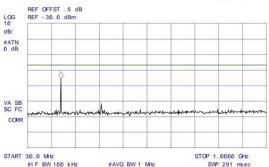
Plot # 2: Receiver Antenna Port Power Conducted Emissions Receive Test Frequency: 450 MHz
