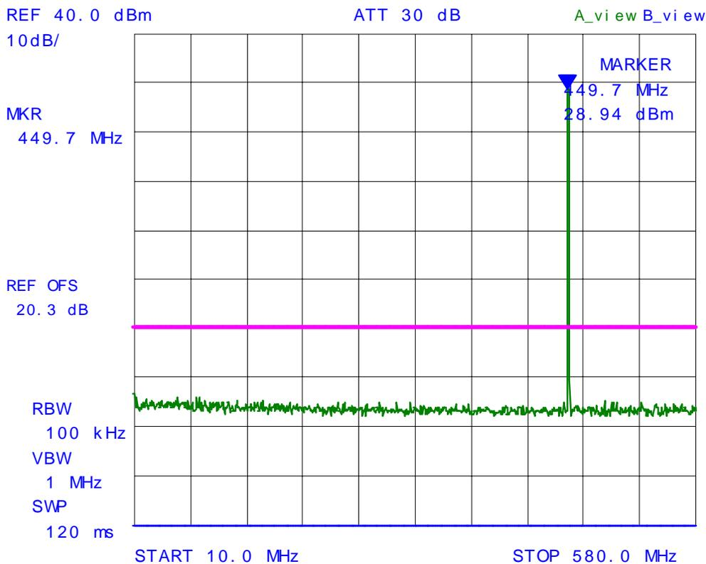
**Plot # 40: Spurious Emissions at Antenna Terminal, Carrier Frequency: 450.05 MHz
