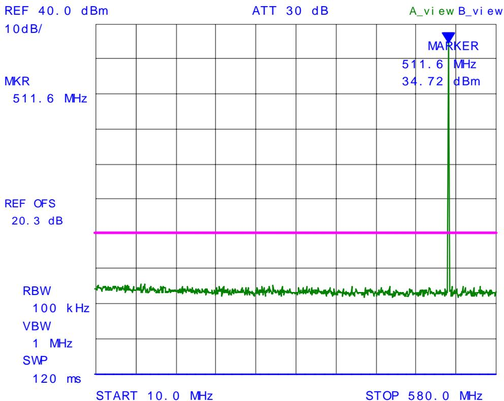
**Plot # 46: Spurious Emissions at Antenna Terminal, Carrier Frequency: 511.95 MHz
