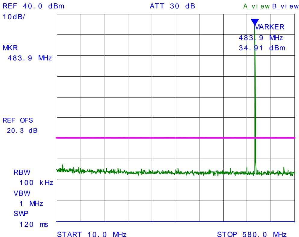
**Plot # 42: Spurious Emissions at Antenna Terminal, Carrier Frequency: 485.05 MHz
