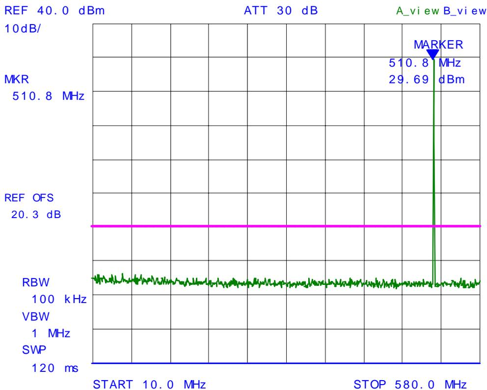
**Plot # 48: Spurious Emissions at Antenna Terminal, Carrier Frequency: 511.95 MHz
