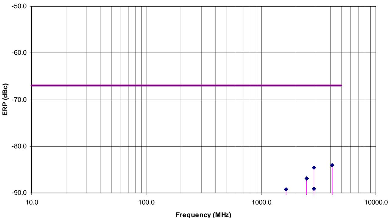
**6.11.5.3. Highest Frequency at High Output Power (Tx Freq: 429.90 MHz, RF Output Power 47 dBm, Modulation: FM with 2.5 kHz Sine Wave Signal, Channel Spacing Setting: 12.5 kHz)**
