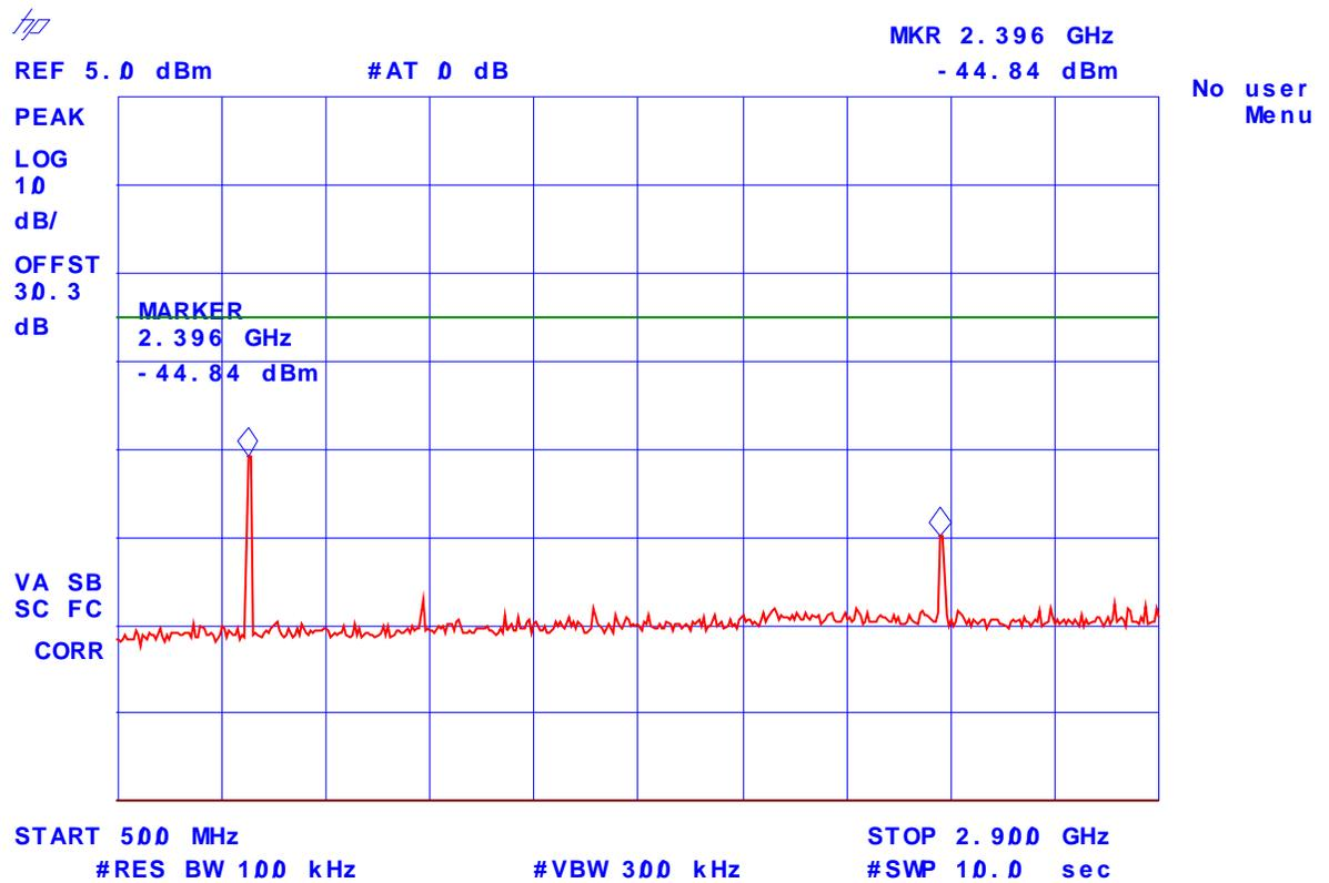
**Plot #33: Transmitter Antenna Power Conducted Emissions**
