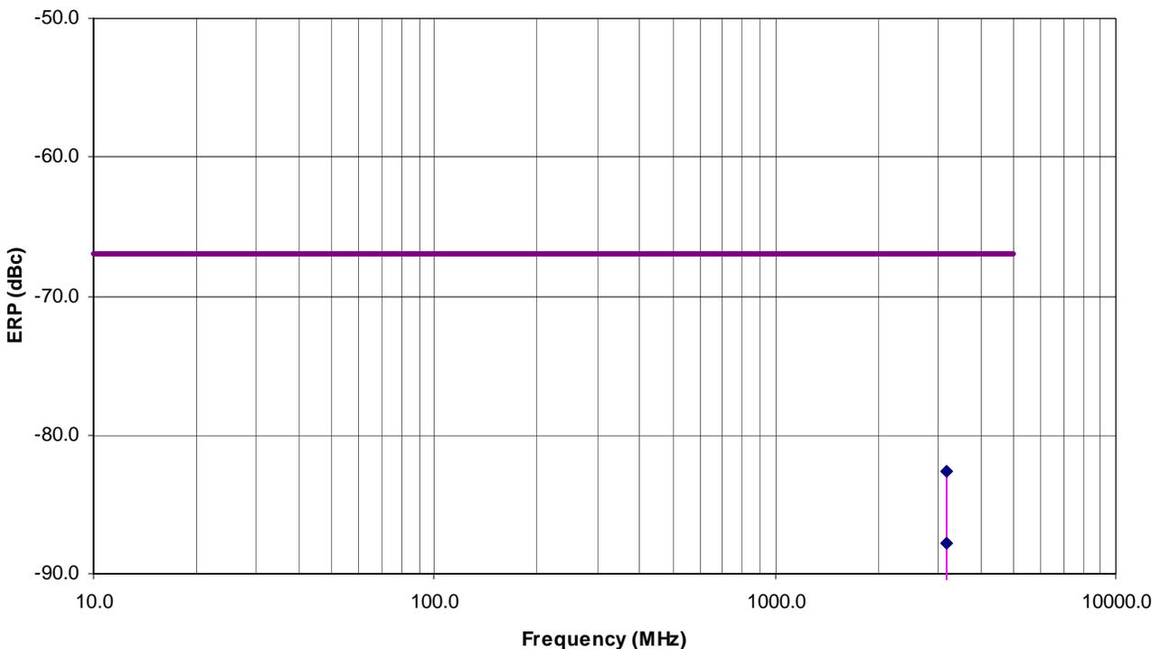
**6.11.5.2. Middle Frequency at High Output Power (Tx Freq: 415.50 MHz, RF Output Power 47 dBm, Modulation: FM with 2.5 kHz Sine Wave Signal, Channel Spacing Setting: 12.5 kHz)**
