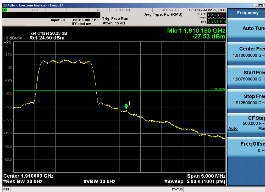
Plot 7-21. Band Edge Plot (PCS CDMA Mode – Ch. 1175)
