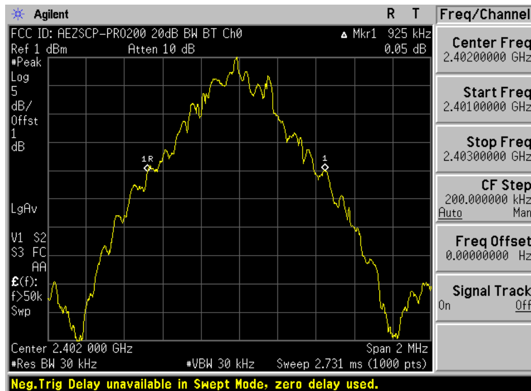
Plot 6-1. 20dB Bandwidth Plot (Bluetooth – Ch. 0)
