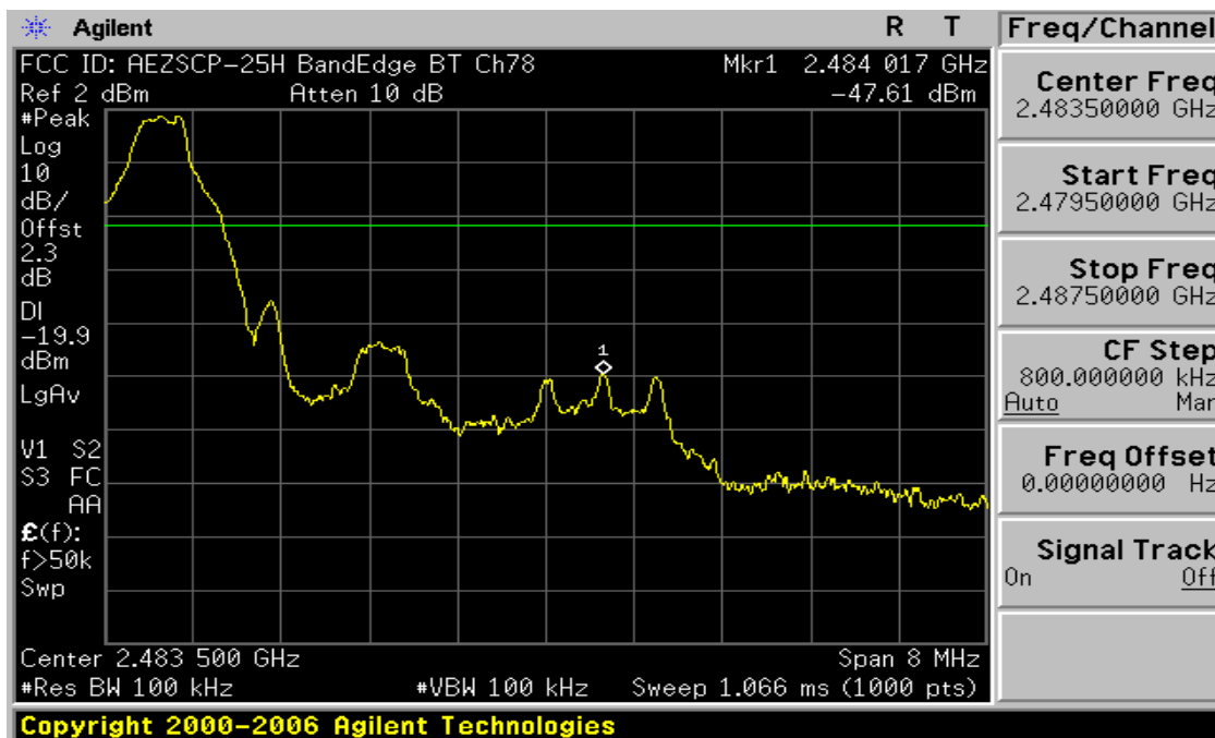
Plot 6-5. Band Edge Plot (Bluetooth – Ch. 78)
