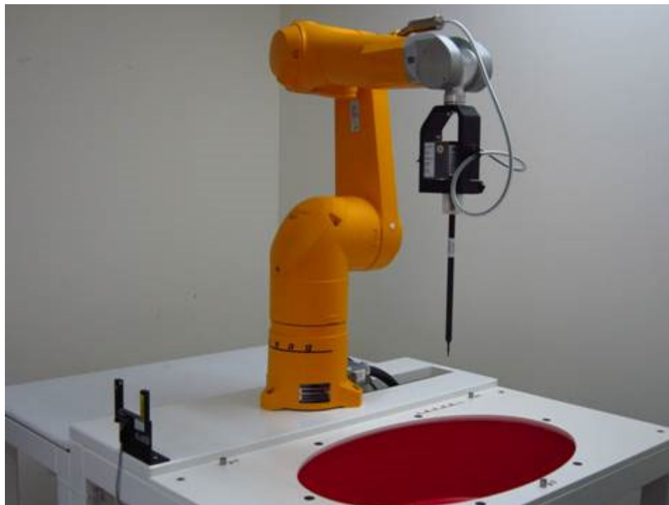
Fig.1 Photograph of the SAR measurement system
