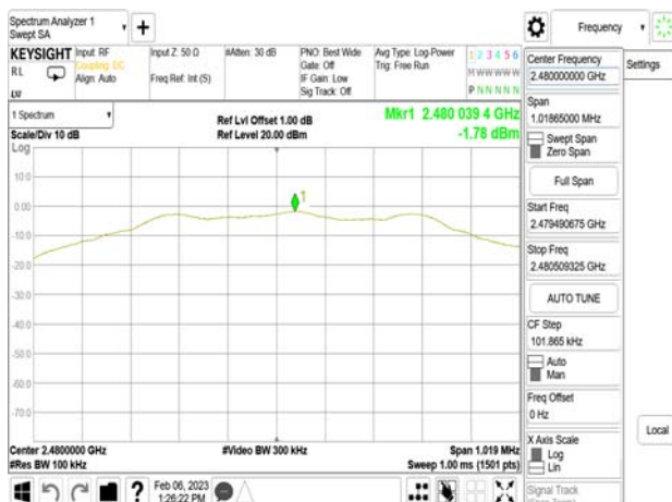
Reference Level_BLE 1M_HighCH39-2480MHz
