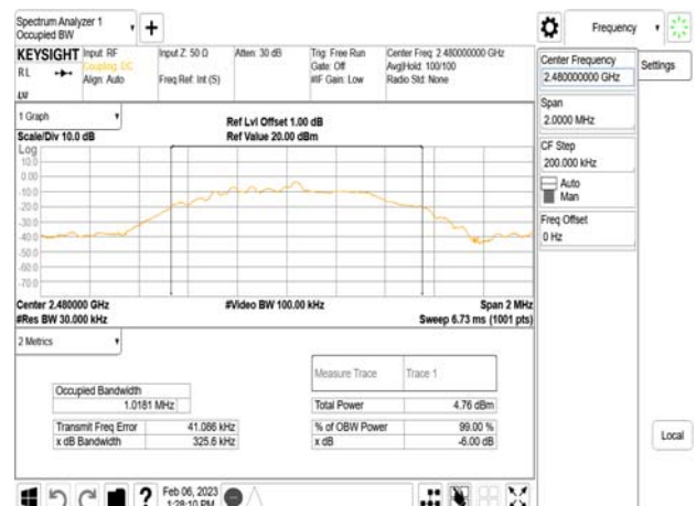
IC OBW_BLE 1M_HighCH39-2480MHz
