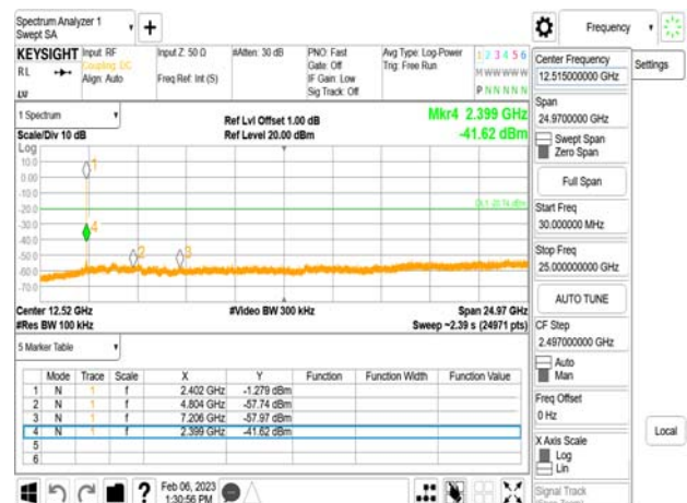
Spurious Emission_BLE 1M_LowCH00-2402MHz
