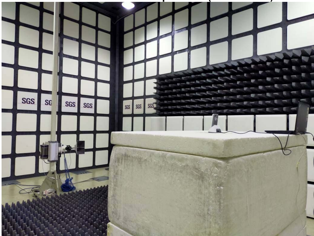
Radiated Emission Set up Photos (Above 1GHz)
