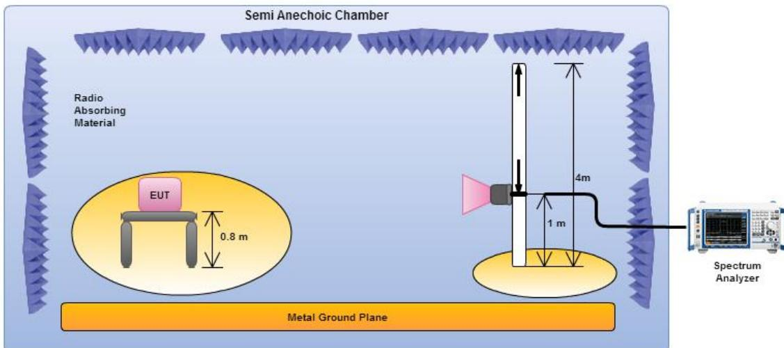
Electric field tests shall be performed in transmitter bandedge emissions using a calibrated horn antenna.
