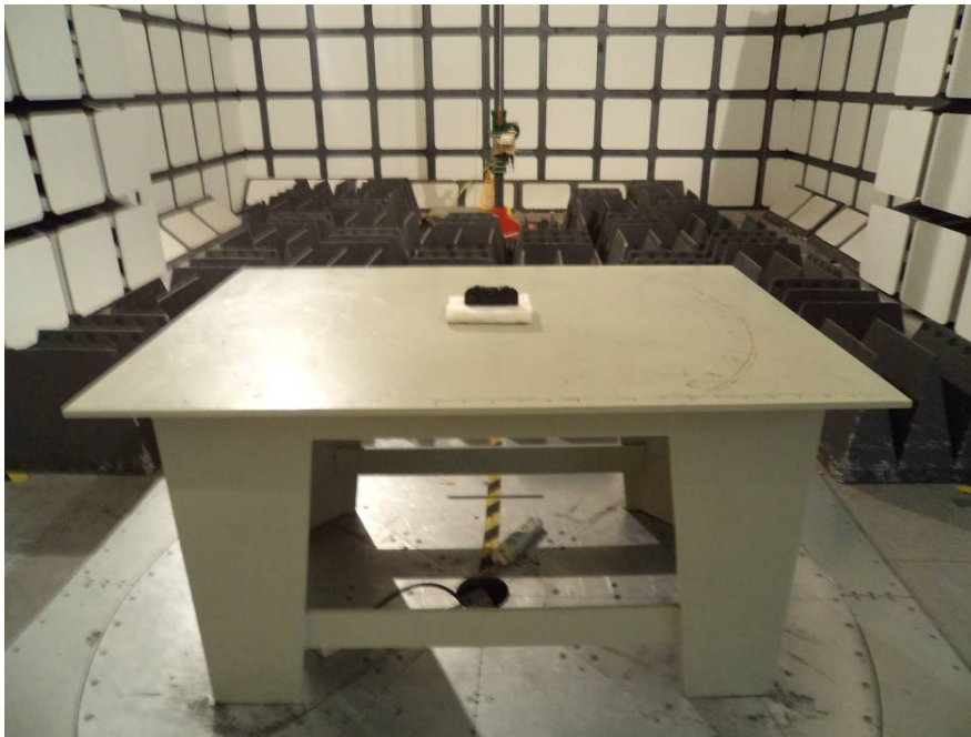
Radiated Emissions View (Above 1 GHz)
