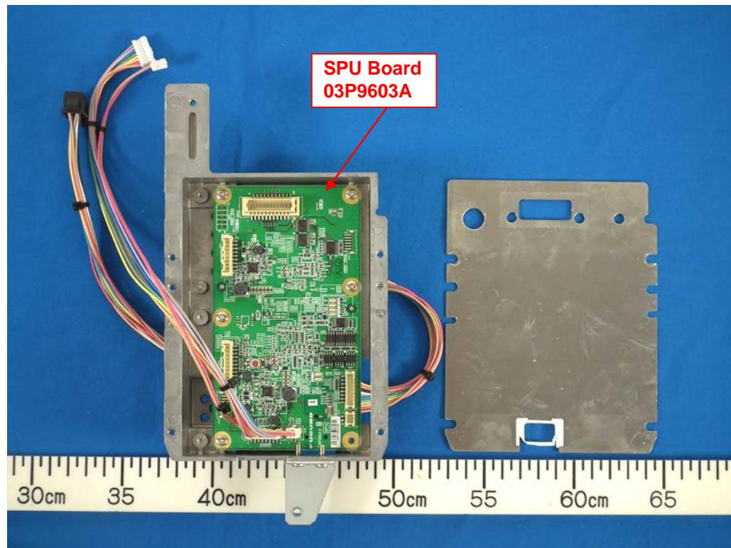
3.15 SPU module (with SPU Board removed)
