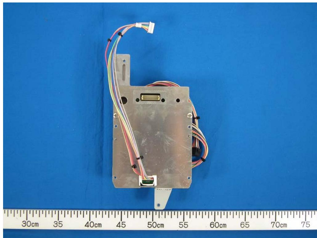
3.14 SPU module (showing SPU Board 03P9603A)
