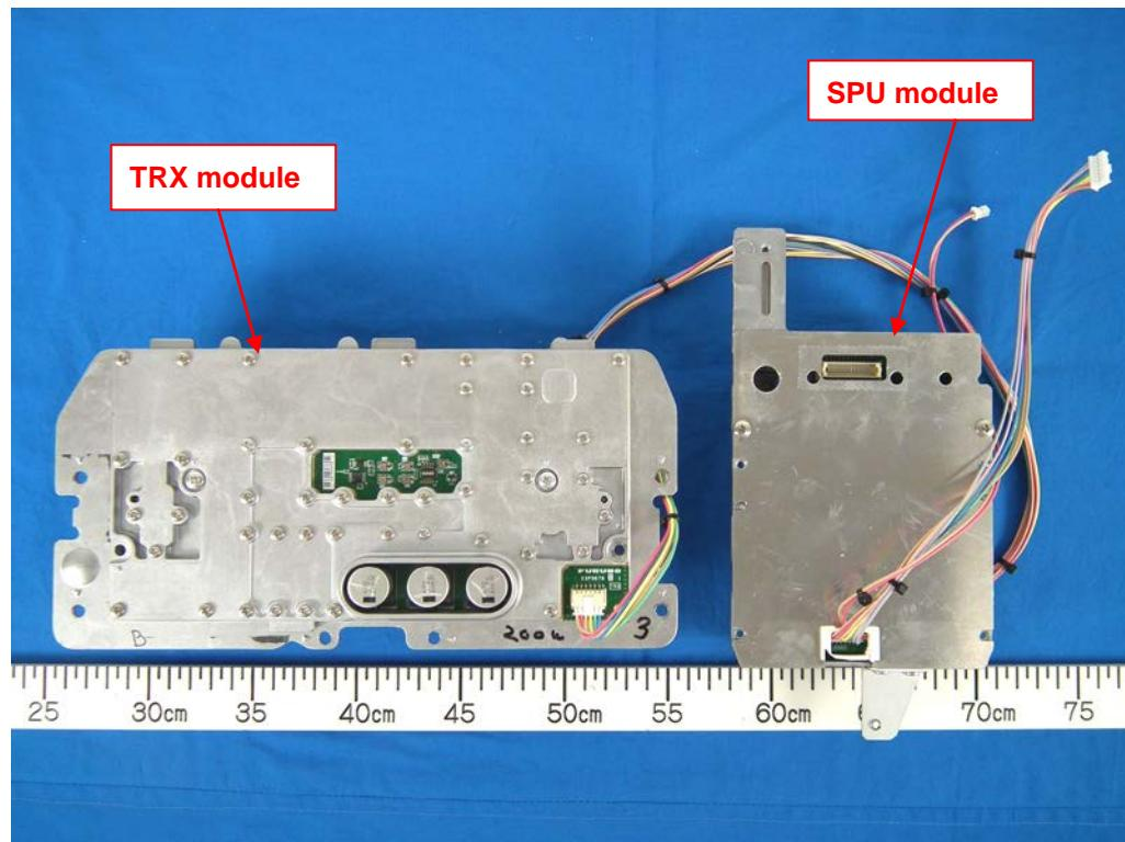
3.8 TRX module (with the shield-cover removed, showing TRX Board 03P9678B)
