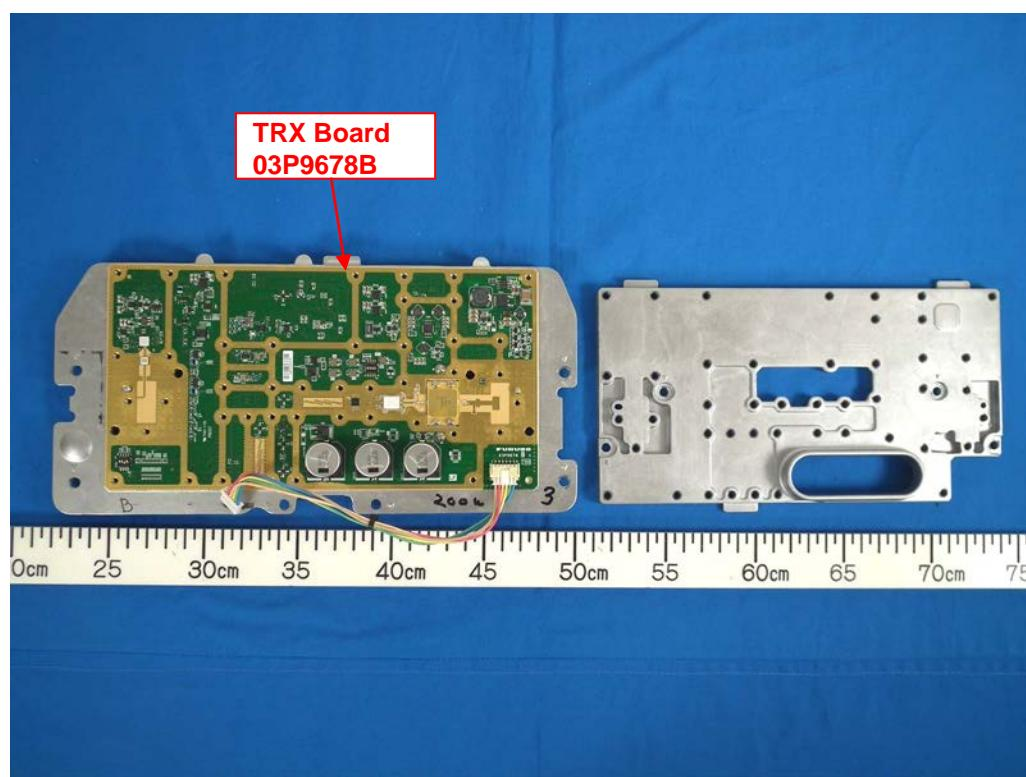
3.9 TRX module (with Circulator removed)
