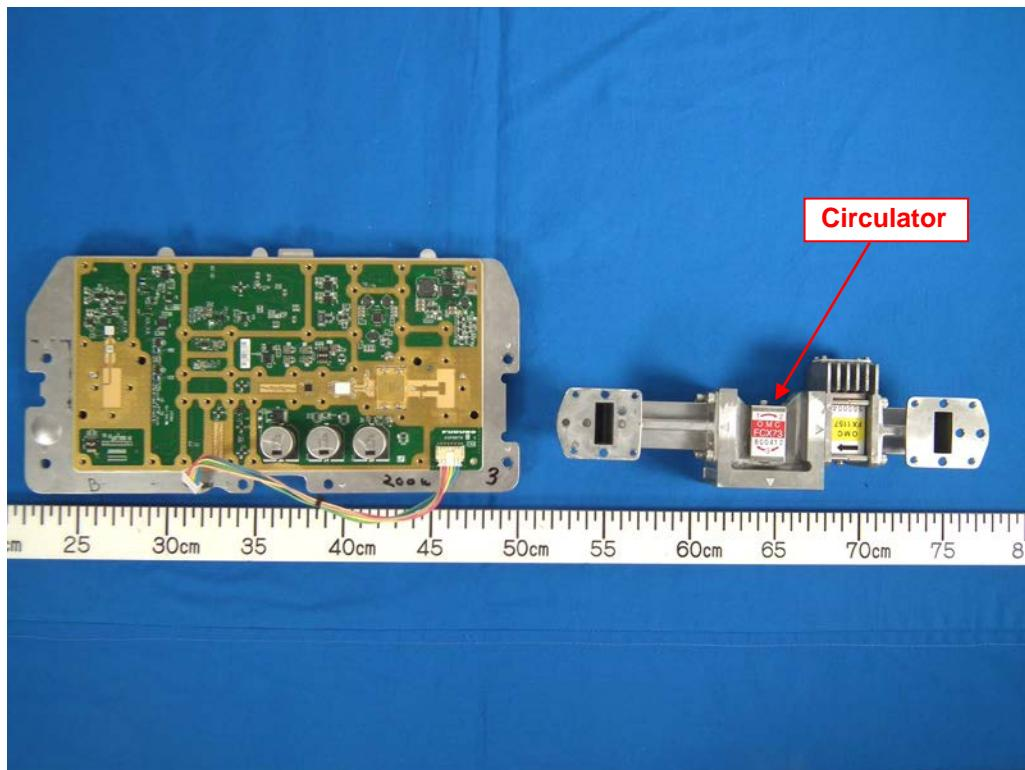
3.10 TRX module (with TRX Board 03P9678B removed)
