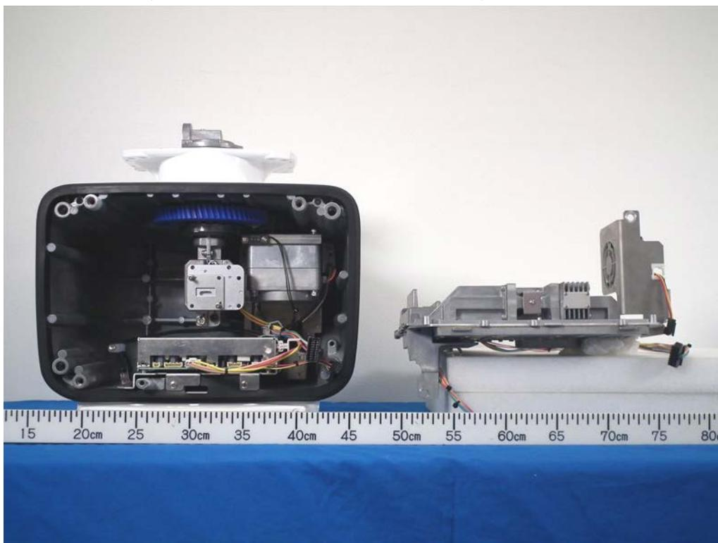
1.3 Inside view (with Power module removed)
