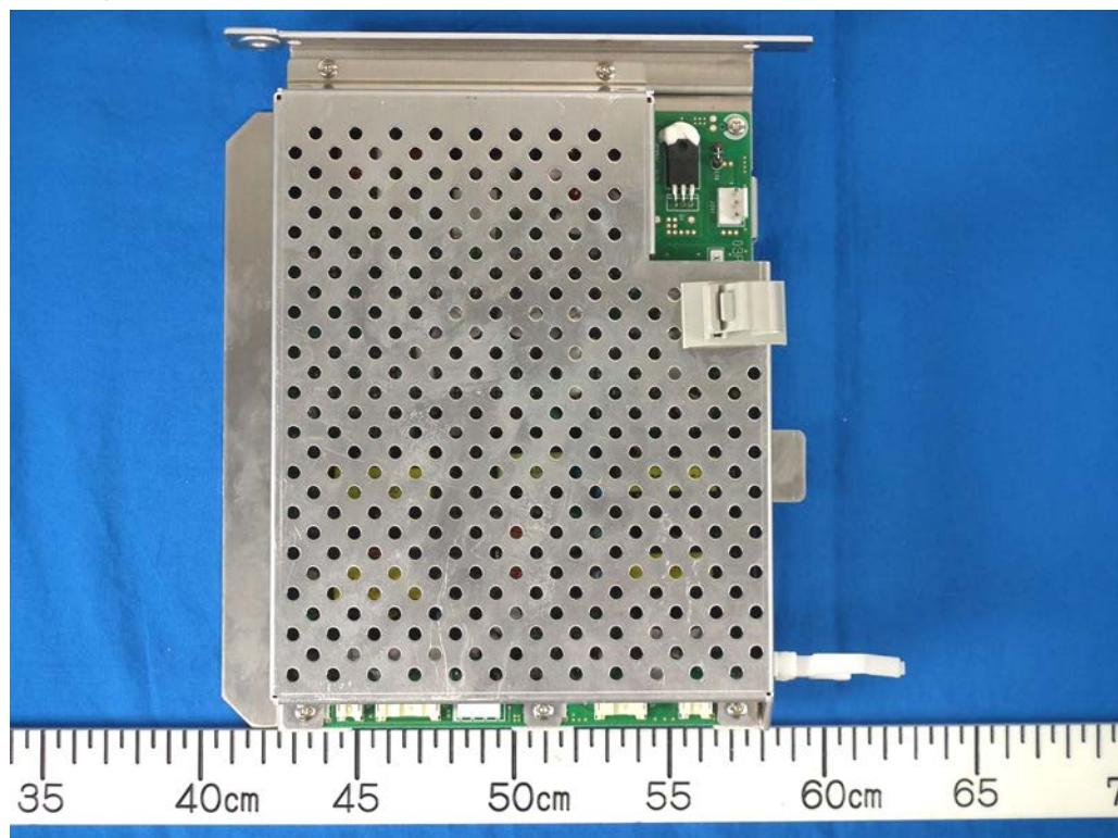
2.2 Top view (with the shield-cover removed, showing PWR Board 03P9679)
