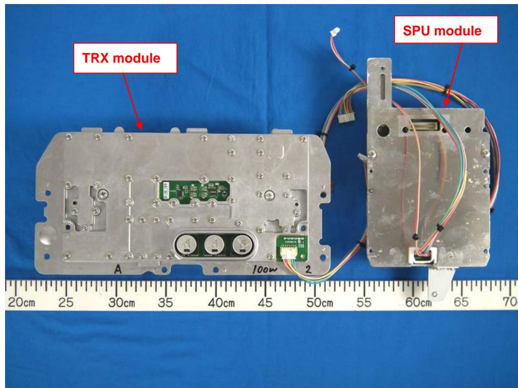
3.8 TRX module (with the shield-cover removed, showing TRX Board 03P9678A)
