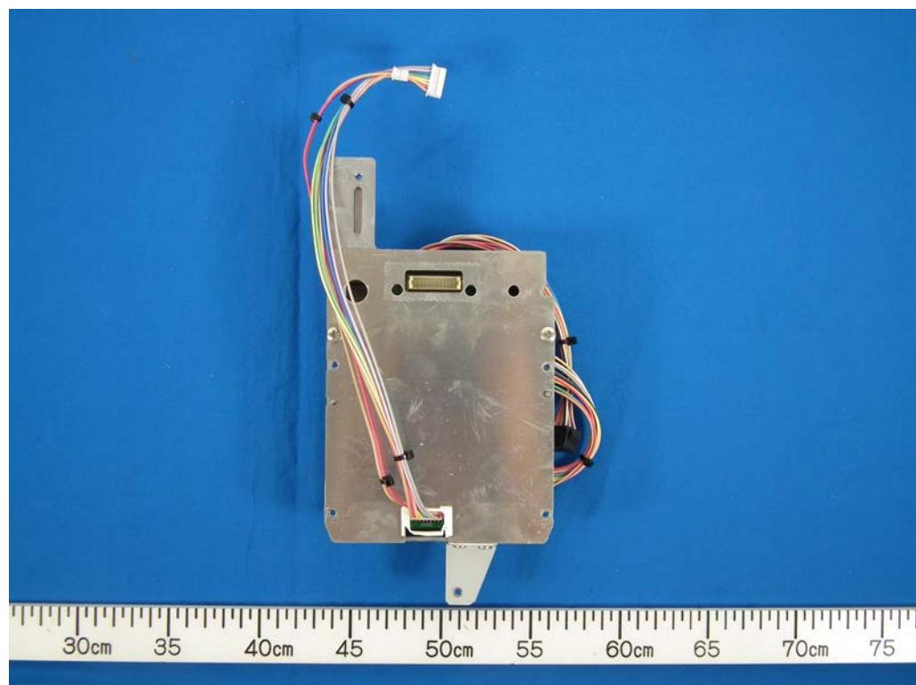
3.14 SPU module (showing SPU Board 03P9603A)
