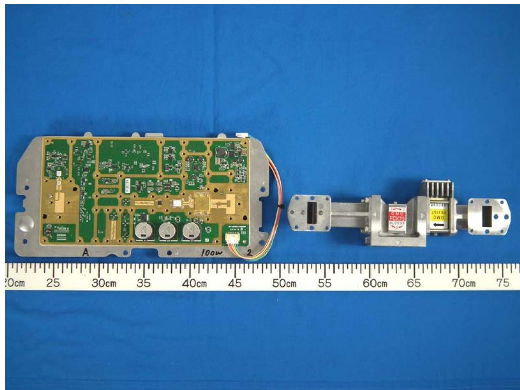
3.10 TRX module (with TRX Board 03P9603A removed)
