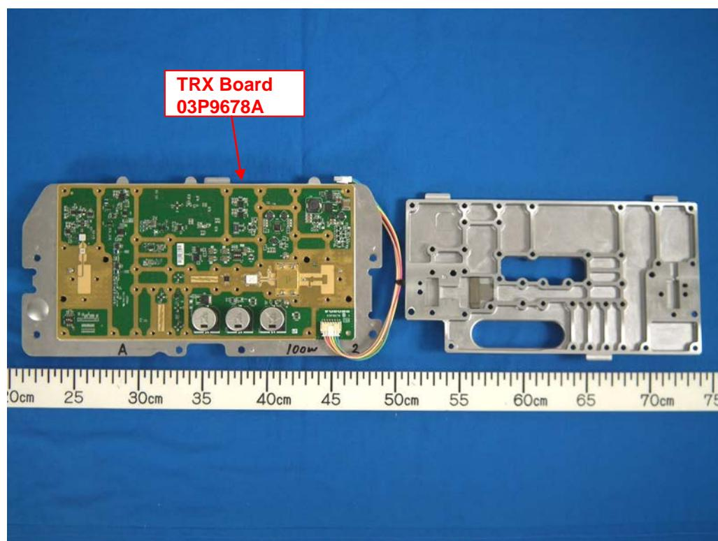
3.9 TRX module (with Circulator removed)
