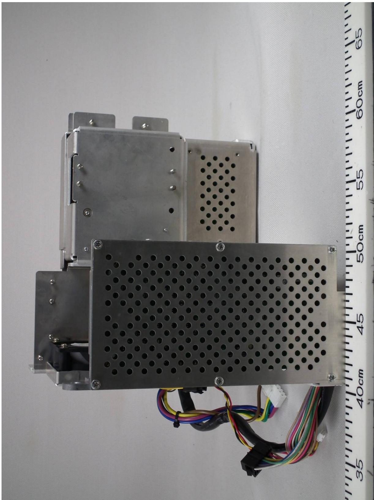
1.13 Transceiver Right side View (with Shield-cover removed, showing SPU Board 03P9598)
