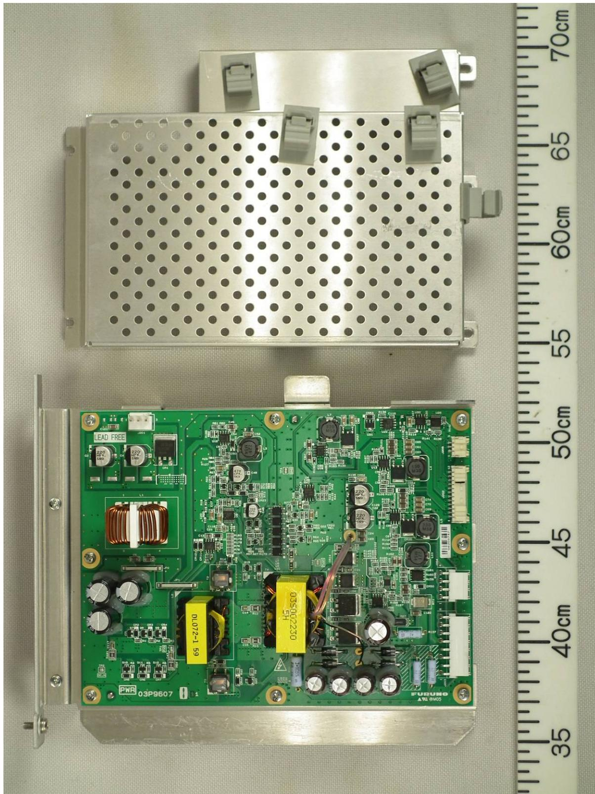
1.8 Power module (with PWR Board 03P9607 removed)
