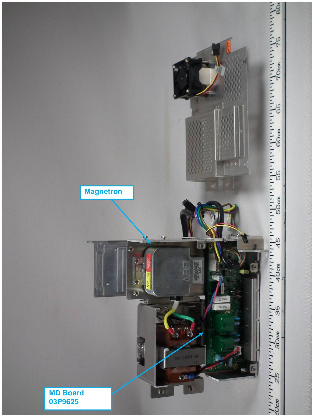
1.18 Transceiver Left side View (showing MD Board 03P9625 and Magnetron)
