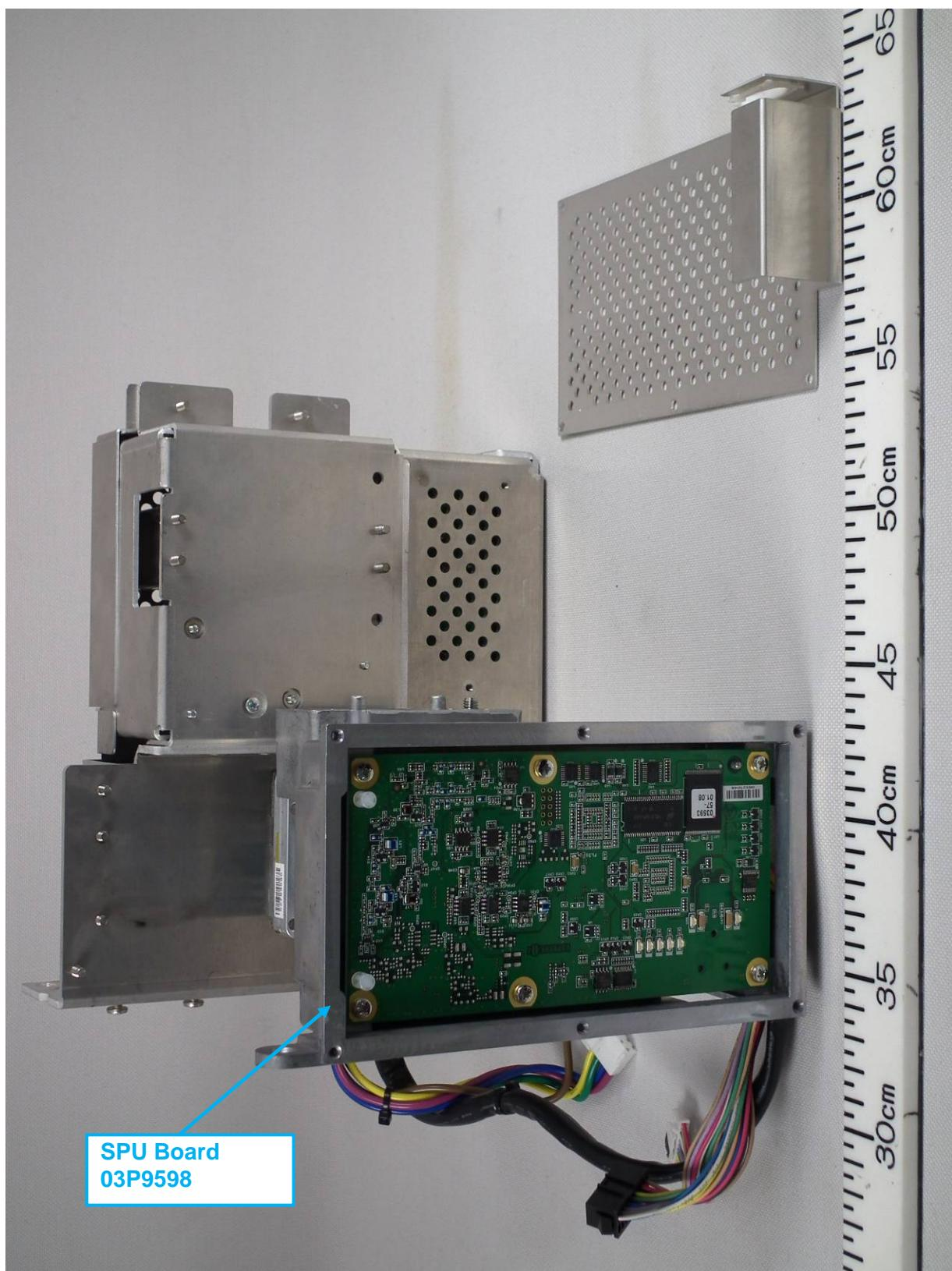
1.14 Transceiver Right side View (with SPU Board 03P9598 removed)
