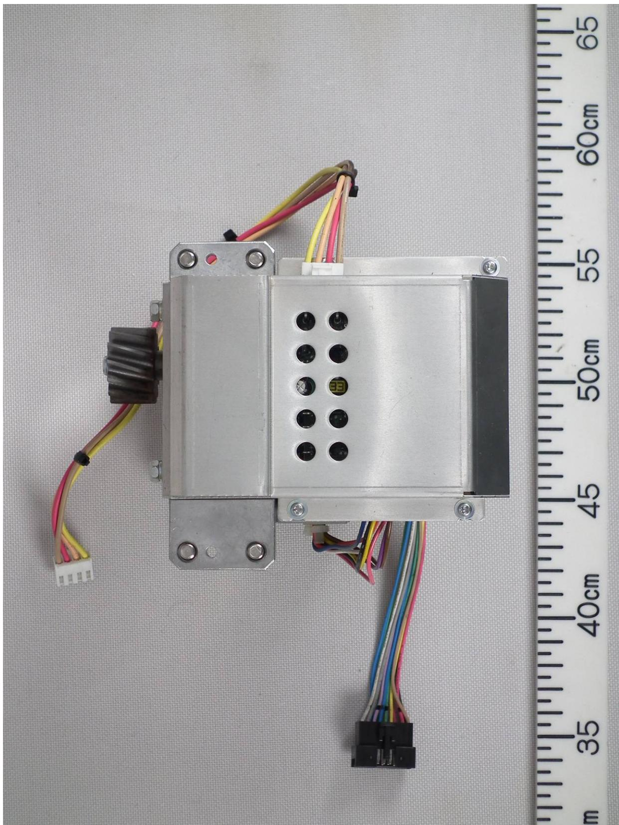
1.22 Motor module Rear side view (with shield cover removed, showing MTR-DRV Board 14DJ003)
