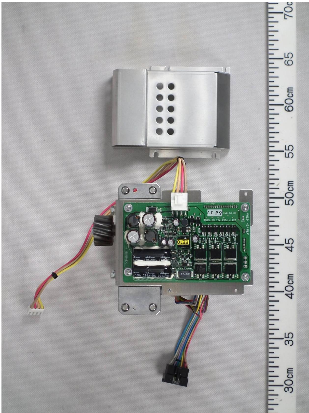
1.23 Motor module Rear side view (with MTR-DRV Board 14DJ003 removed)
