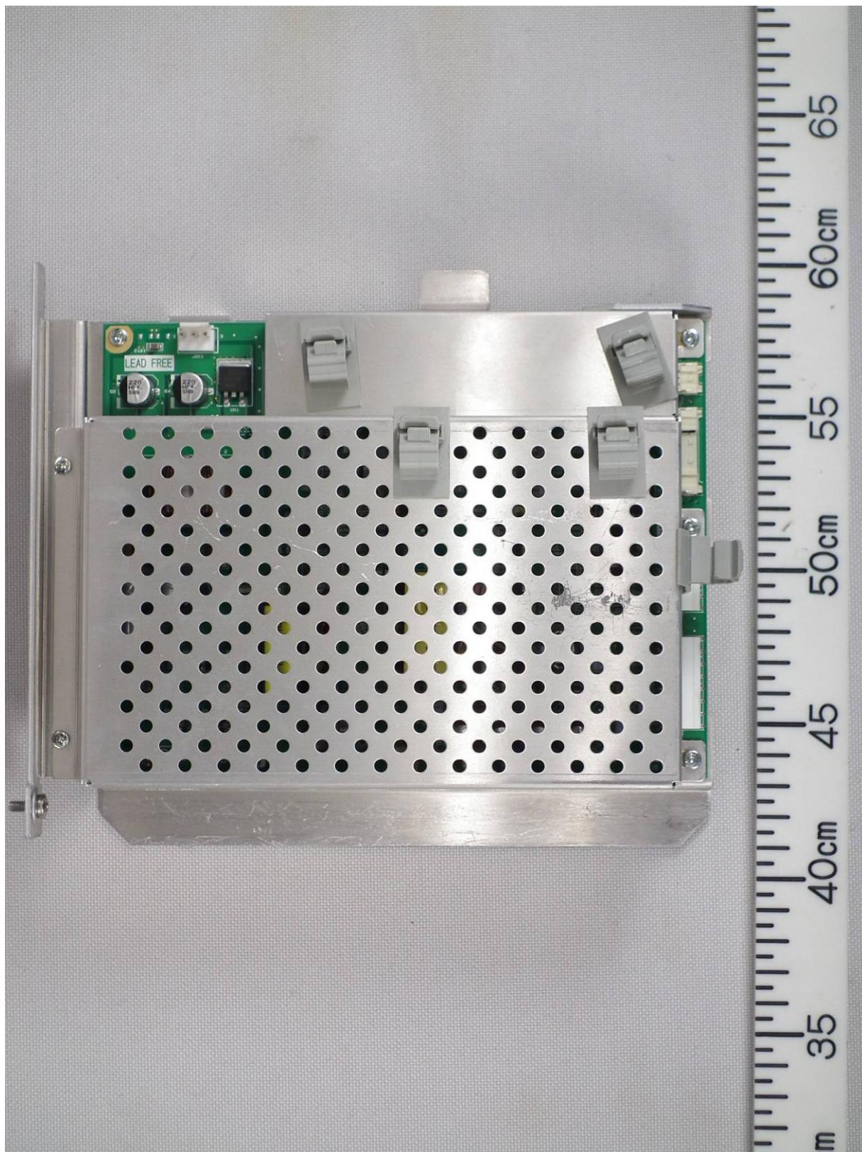
1.7 Power module (with Shield-cover removed, showing PWR Board 03P9607)
