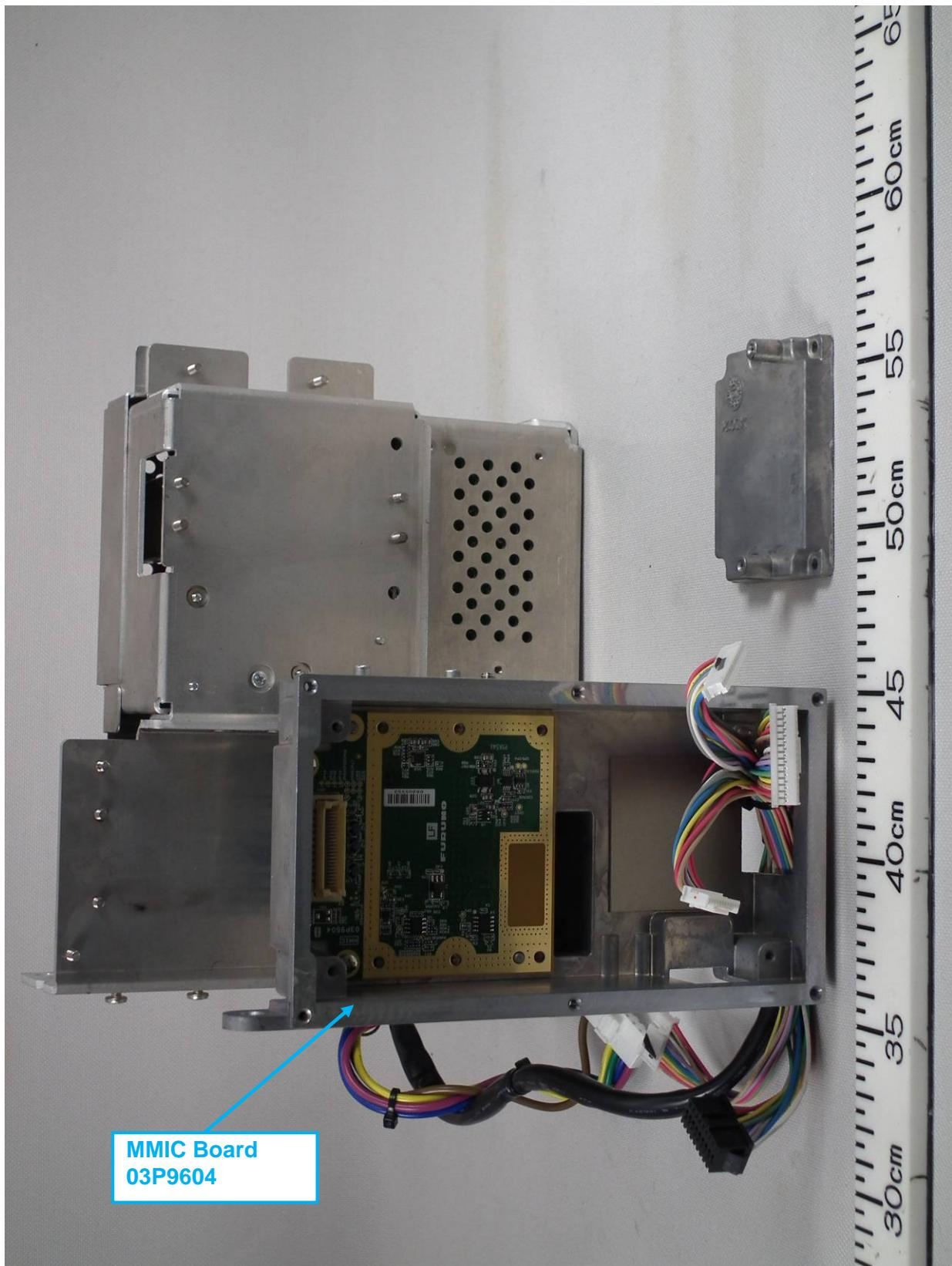
1.16 Transceiver Right side View (with MMIC Board 03P9604 removed)
