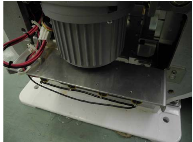
Bottom of the enclosure (ingress of water found around the drain hole. Water drops are indicated by the red arrows.) (with Transceiver removed)
