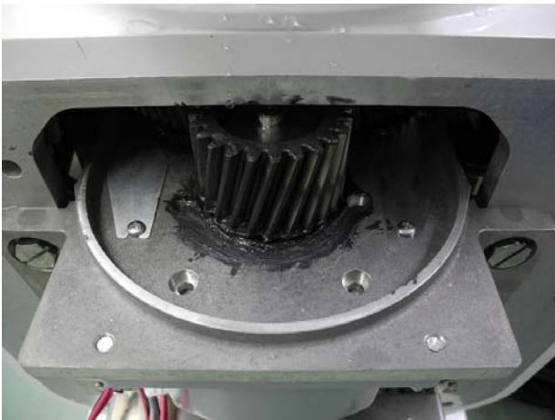
Bottom of the enclosure (ingress of water found around the drain hole. Water drops are indicated by the red arrows.) (with Transceiver removed)
