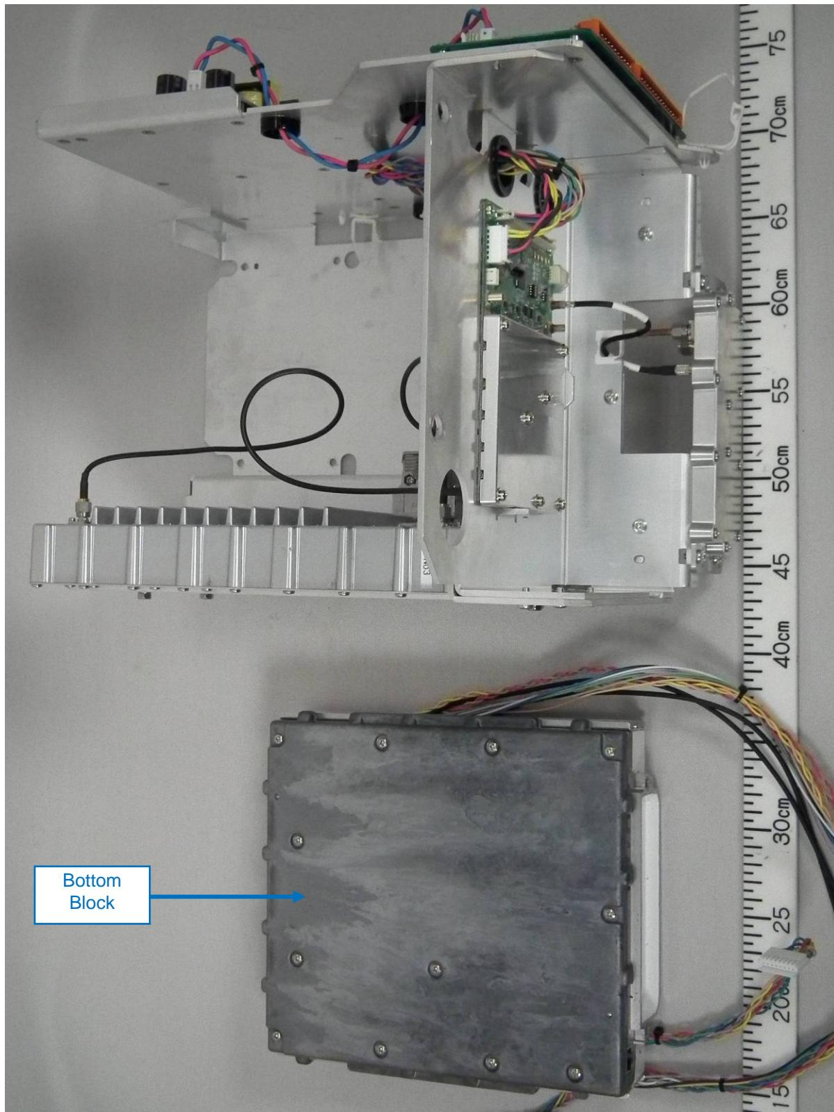
1.1.9 Back of Bottom Block (with base plate opened, showing SPU (SSD) Board 03P9546)
