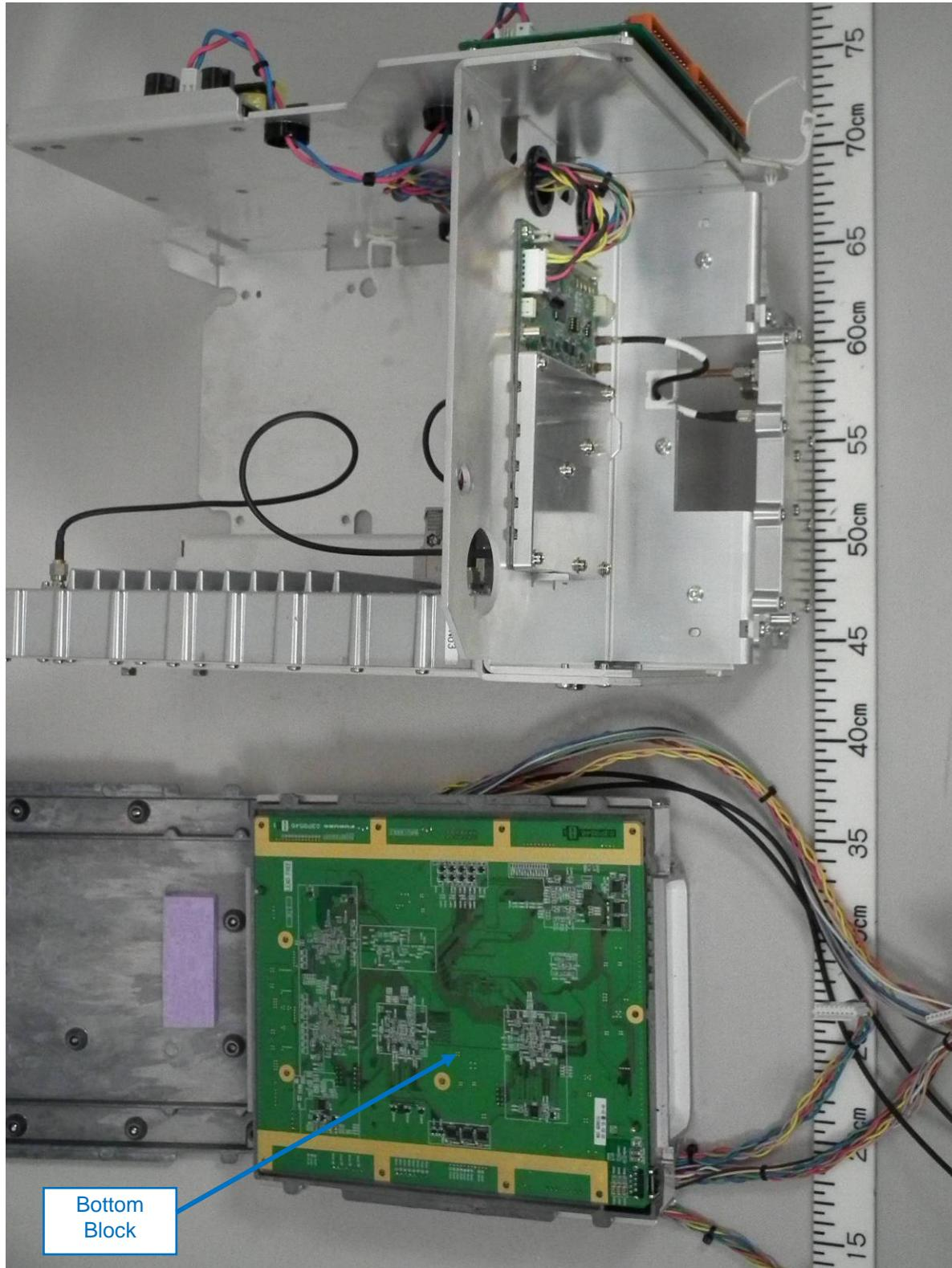
1.1.10 Bottom Block (with SPU (SSD) Board removed)
