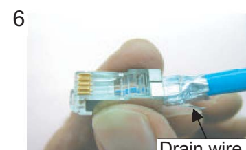
Insert the cable into the modular plug so that the folded part of the shield enters into the plug housing. The drain wire should be located on the tab side of the jack.
