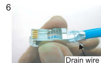
Insert the cable into the modular plug so that the folded part of the shield enters the modular plug. The drain wire must be on the tab side of the jack.
