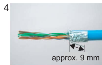
Fold back drain wire and cut it, leaving 9 mm.
