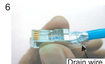
Insert the cable into the modular plug so that the folded part of the shield enters the modular plug. The drain wire must be on the tab side of the jack.
