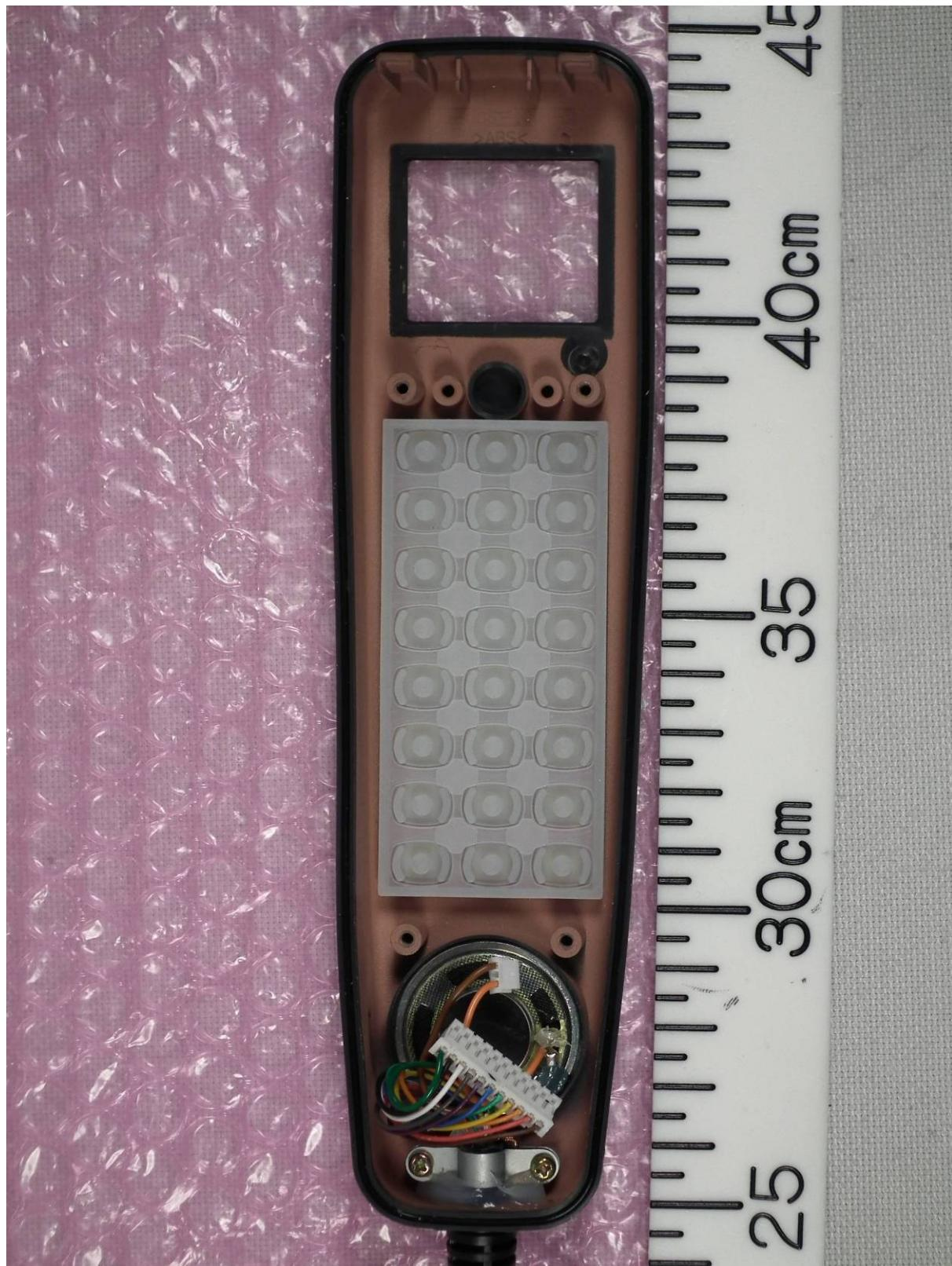
3.6 Handset Hanger Inside View (with Top Cover opened, showing TB Board 05P0798 Front side)
