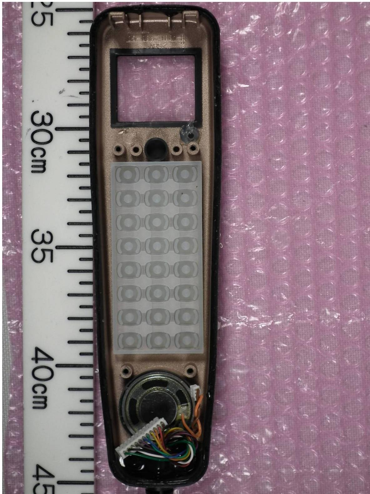
4.6 Handset Hanger Inside View (with Top Cover opened, showing TB Board 05P0798 Front side)
