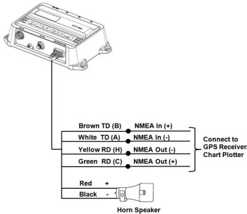
The NMEA 0183 wire should be connected to a compatible NMEA 0183 device as shown in the table below:
