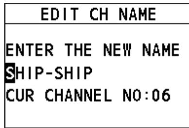
Step 5 Press the **Menu/DSC** control to save the new channel name and return to the previous screen.
