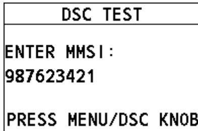
Step 3 Press the **Menu/DSC** control to send the DSC test call.
