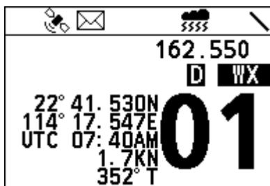
In weather mode, you can rotate the Menu/DSC to select a NOAA channel to monitor. What you selected would be marked as last used weather channel.
