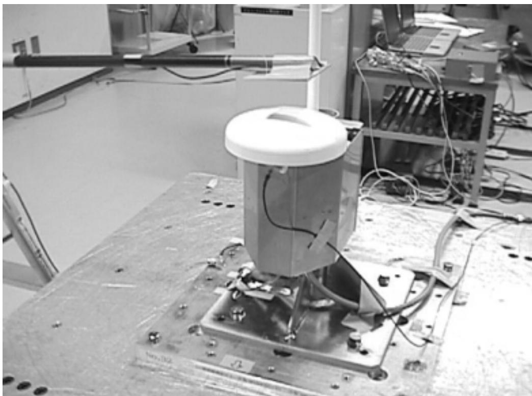
9.13 For Rain test - Combined Antenna GVA-100,
