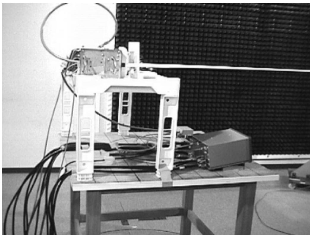
9.9 For Vibration test - Transponder FA-100
