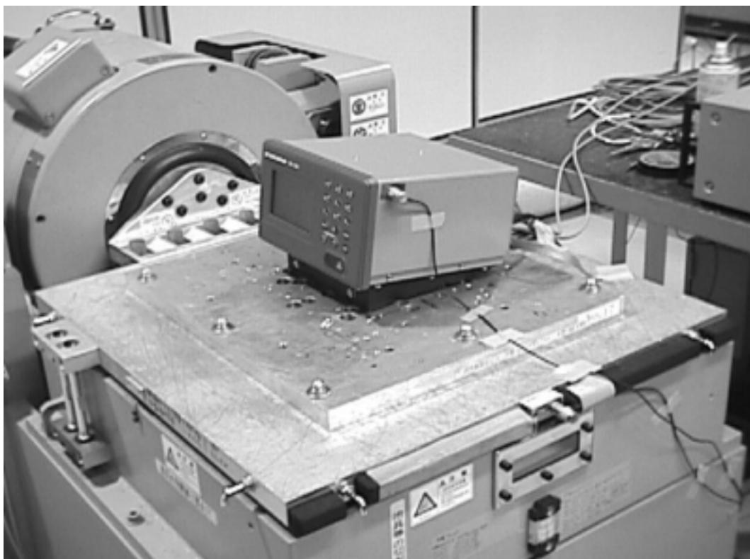
9.10 For Vibration test - Connection Box CB-100
