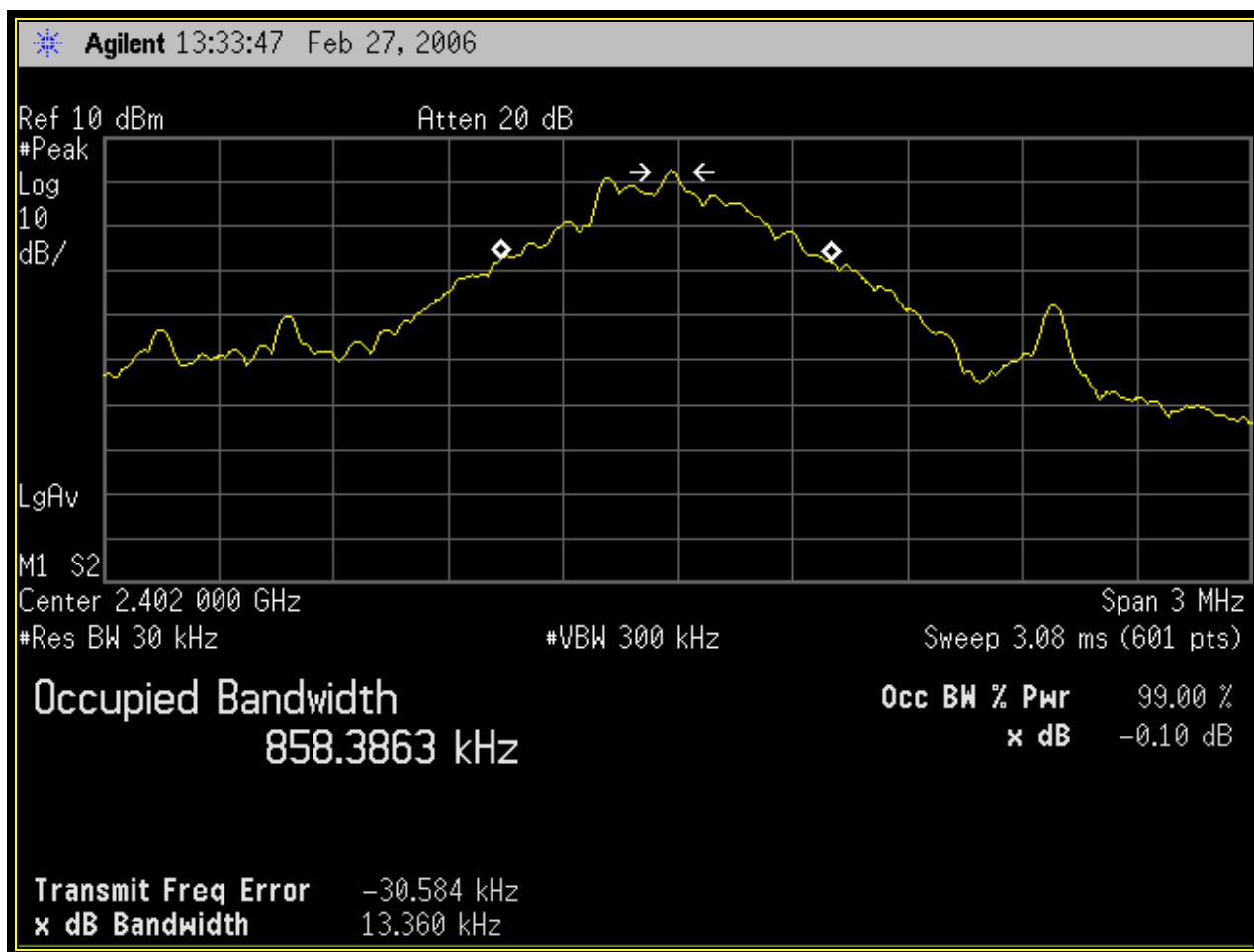
Plot 6-1: 20 dB Bandwidth Channel 0
