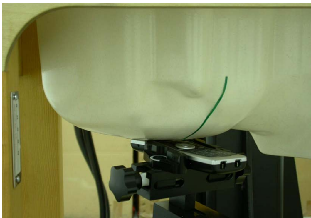
Measurement Position of Right-Cheek (RC) with Handset
