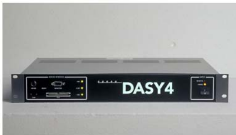
Fig. 7 DASY4 Measurement Server
