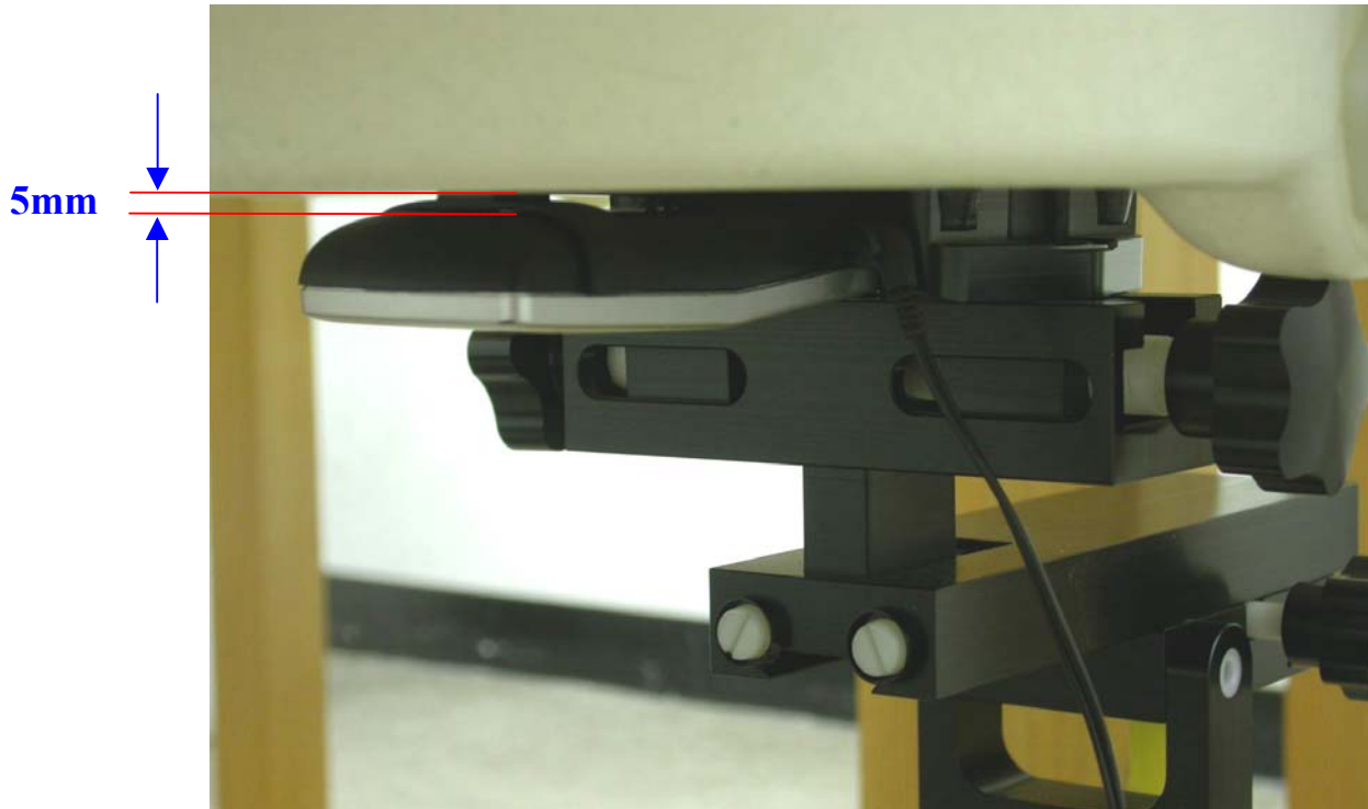
Measurement Position of Rear-UP with Handset
