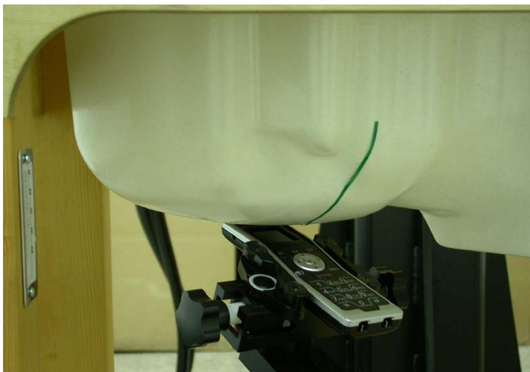
Measurement Position of Right-Tilt (RT) with Handset
