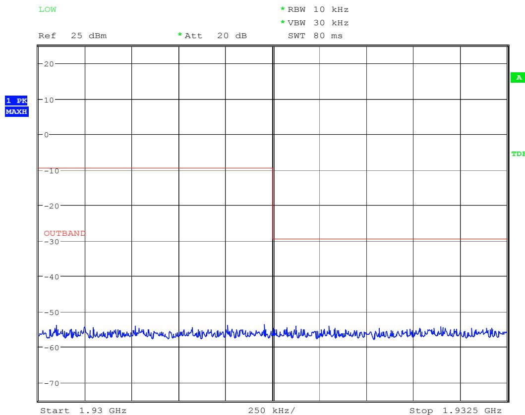
**Out-of-band Unwanted Emissions: CH F<sub>L</sub>.**
