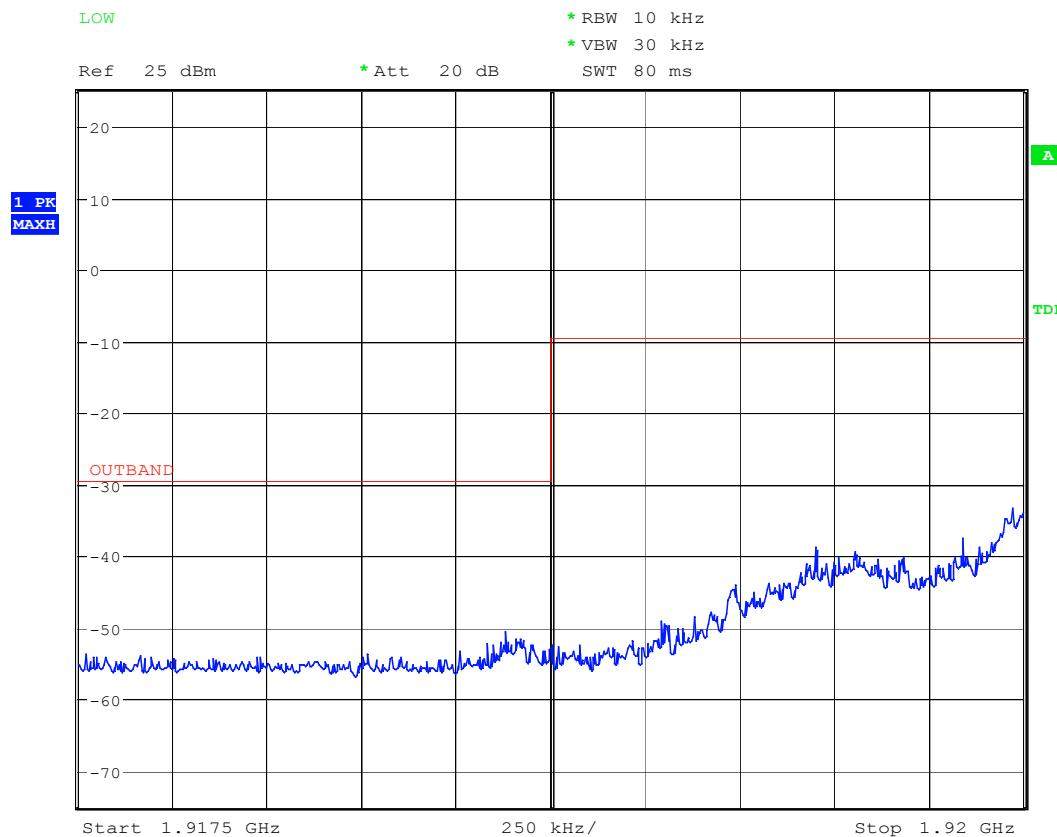
**Out-of-band Unwanted Emissions: CH F<sub>L</sub>.**
