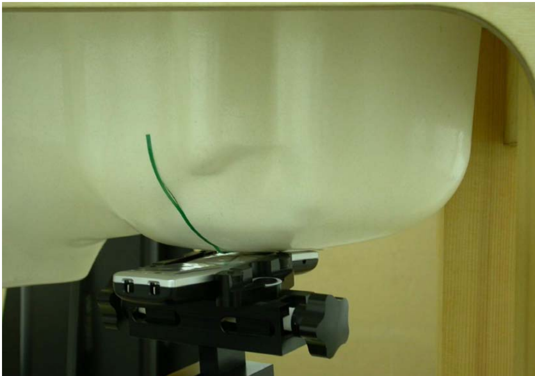
Measurement Position of Left-Cheek (LC) with Handset
