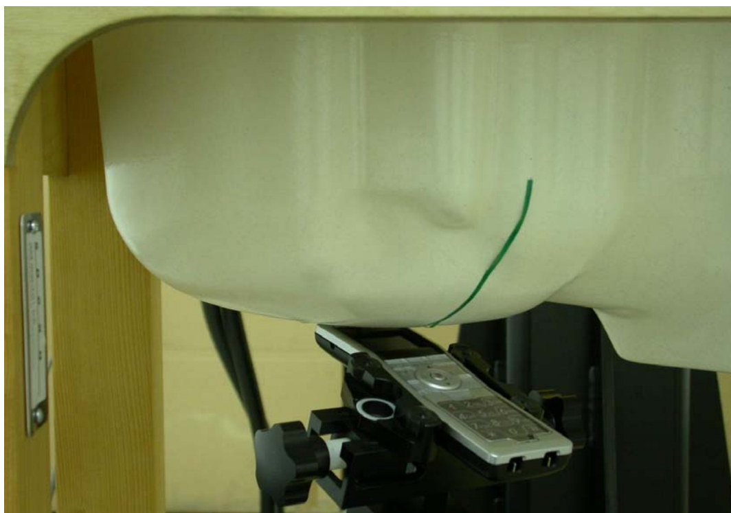
Measurement Position of Right-Tilt (RT) with Handset
