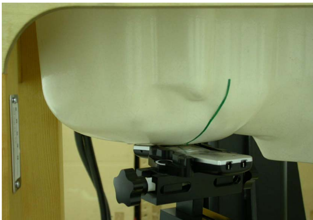
Measurement Position of Right-Cheek (RC) with Handset
