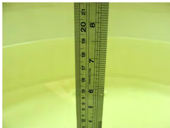
Fig 6.2 Photo of Liquid Height for Body SAR
