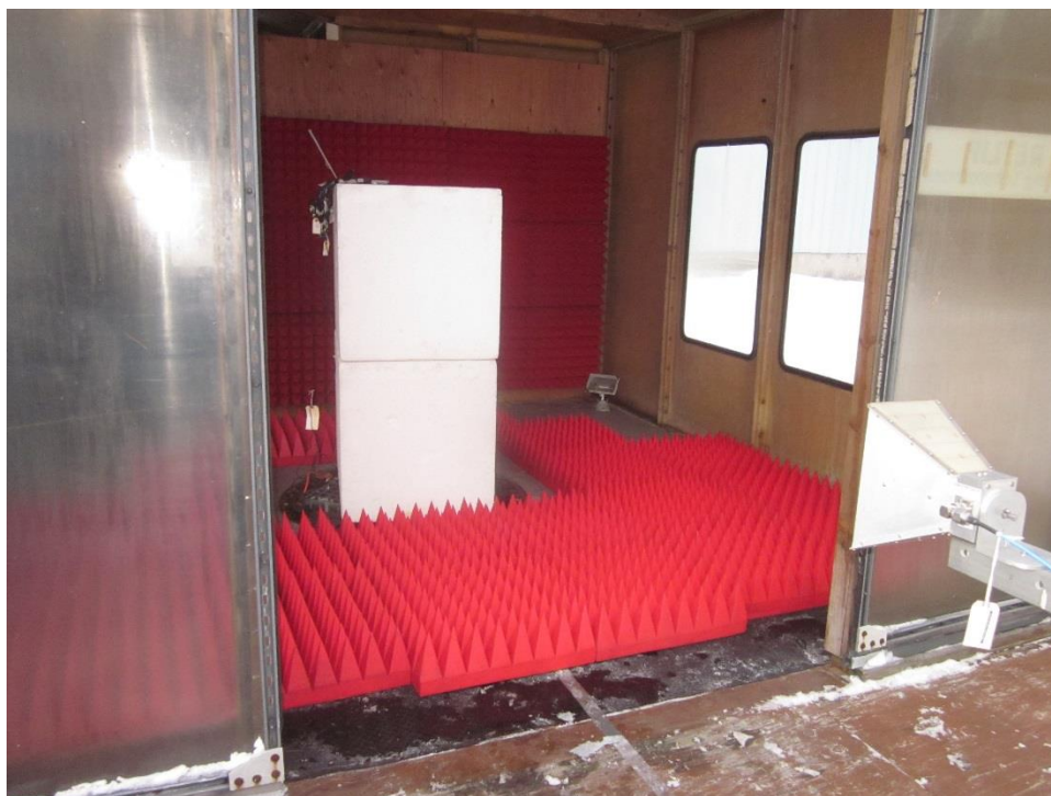
Horizontal Polarization, 1- 18 GHz, Double Ridge Guide
