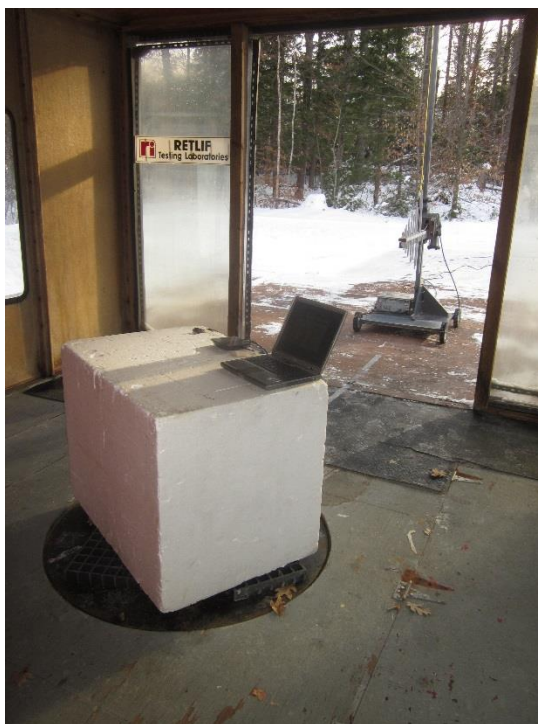
Vertical Polarization, 200 MHz - 1 GHz, Log Periodic
