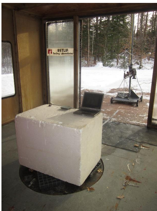
Vertical Polarization, 30 MHz – 200 MHz, Biconical Antenna
