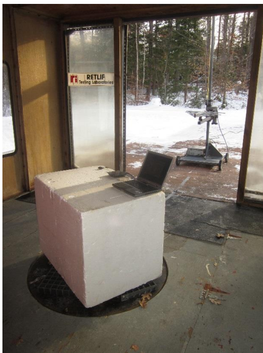
Horizontal Polarization, 200 MHz - 1 GHz, Log Periodic
