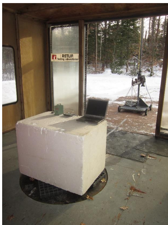
Vertical Polarization, 30 MHz – 200 MHz, Biconical Antenna
