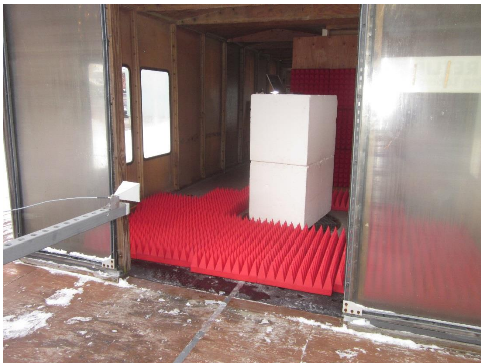
Horizontal Polarization, 18- 26 GHz, High Gain Horn
