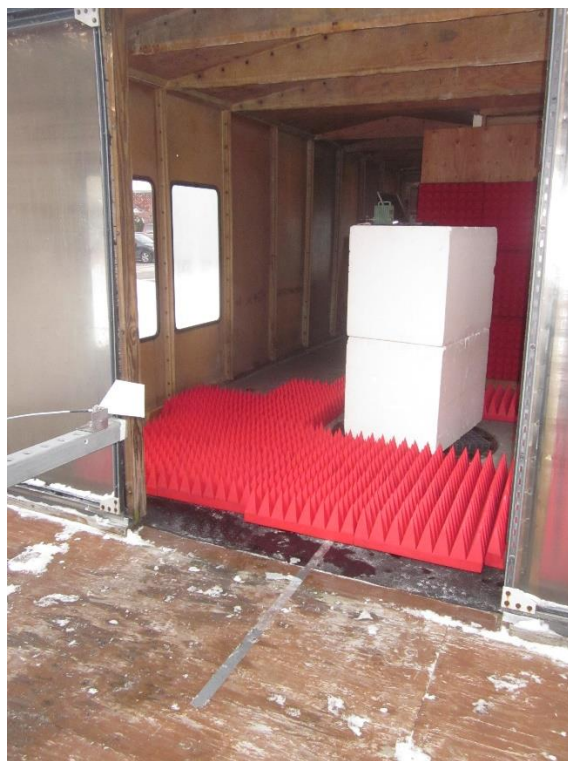
Horizontal Polarization, 18- 25 GHz, High Gain Horn
