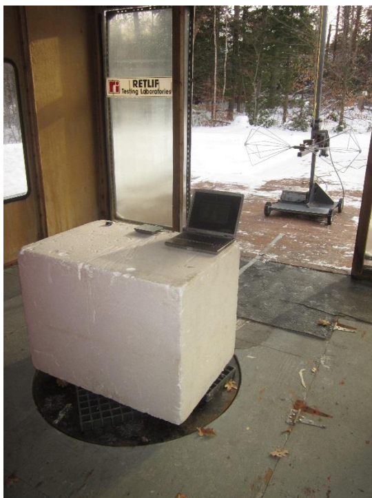
Horizontal Polarization, 30 MHz – 200 MHz, Biconical Antenna
