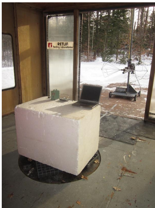
Horizontal Polarization, 30 MHz – 200 MHz, Biconical Antenna
