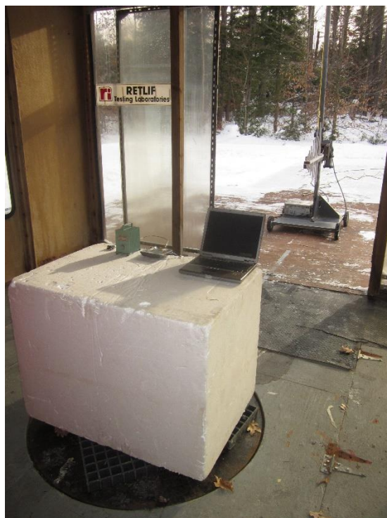
Vertical Polarization, 200 MHz - 1 GHz, Log Periodic
