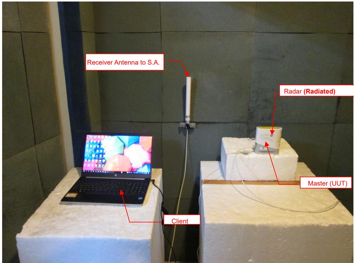
For Slave without radar detection setup
