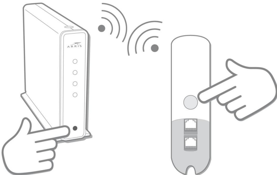
The LED on the X5 flashes green quickly when it has paired successfully with the gateway.
