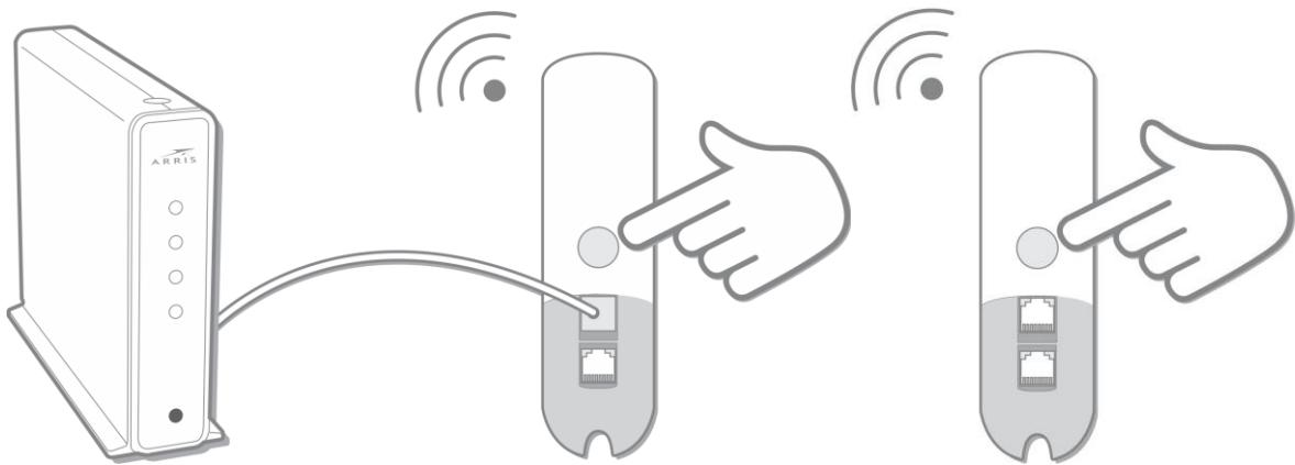
The second X5 will be automatically configured with the same Wi-Fi settings as the first X5; this will take a few moments. The LED on the second X5 flashes green quickly when the two units pair successfully.
