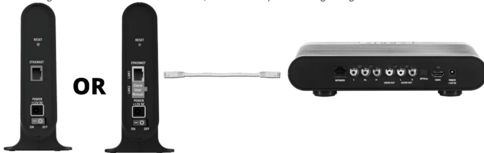
2. Connect the power adapter to the VAP, plug the adapter into a wall outlet and set the Power switch to the ON position. You'll see the power LED on the unit's front panel light green, indicating the unit is powered.
