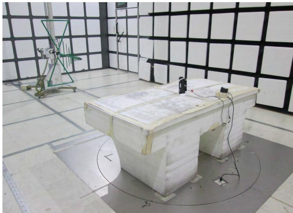
**Test Configuration: 1GHz~40GHz**
