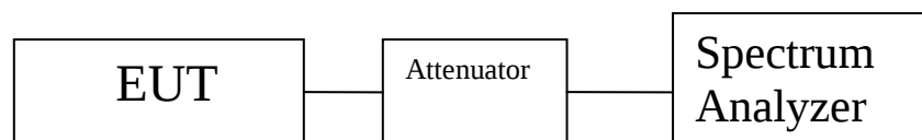
Figure 3. Block Diagram, Conducted Spurious Emissions Test Setup
