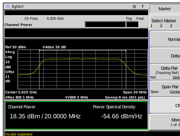
Plot 28. RF Power Output, Channel 165, 802.11ac 20 MHz, SISO
