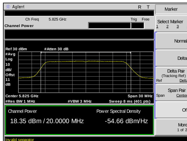
Plot 40. RF Power Output, Channel 165, 802.11n 20 MHz, SISO
