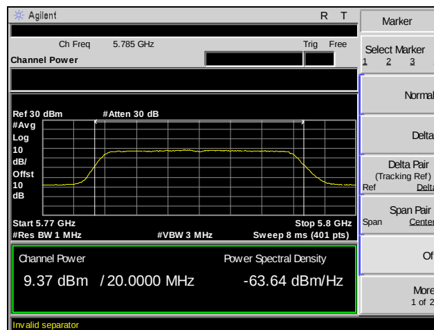
Plot 36. RF Power Output, Channel 157, 802.11n 20 MHz, MIMO
